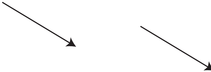
Figure 5-3. If vectors have the same magnitude and direction, they are the same. Position doesn't matter.
