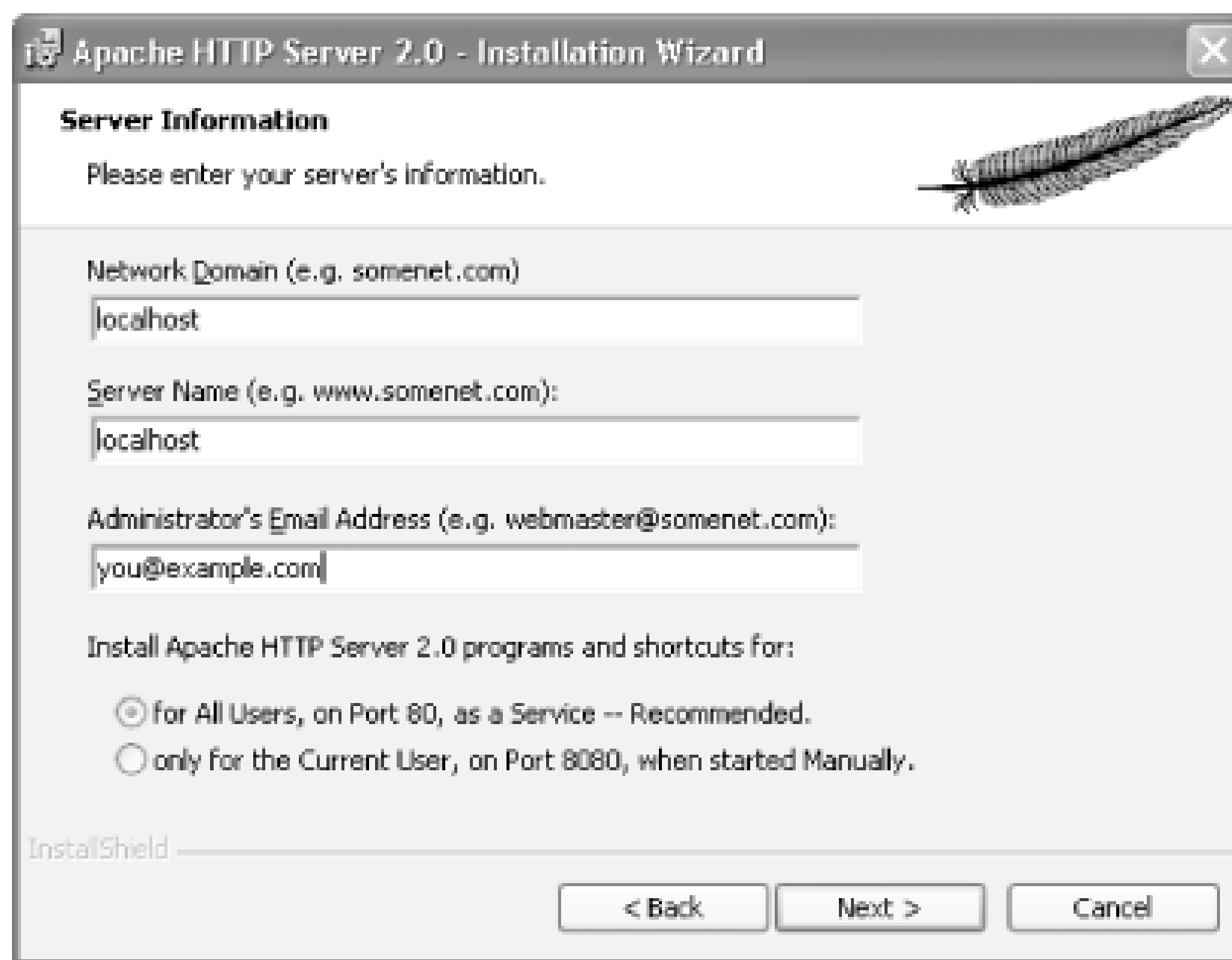
Figure A-17. Entering server information
