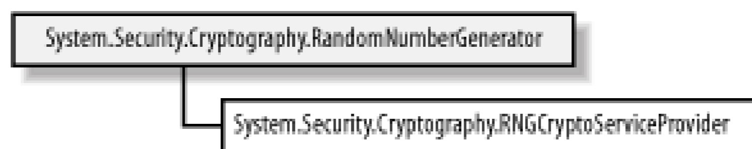
Figure 17-3. The .NET Framework class hierarchy for random number generators
