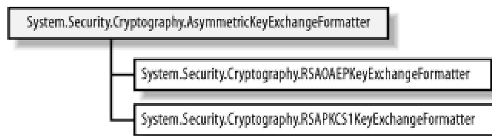
Figure 17-5. The .NET Framework class hierarchy for key exchange formatting
