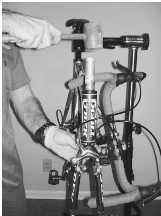
Remove the fork by gently tapping on the steerer tube with a rubber mallet.
