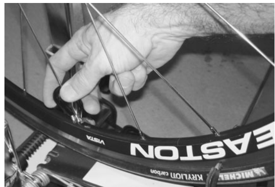
Make small adjustments when truing a wheel, turning the spoke nipple one-quarter to one-half turn at a time using a spoke wrench.
