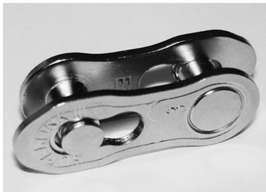
Using a master link instead of a connecting pin makes it easy to install and remove a chain.
