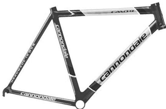
Traditional tubing is round in cross section. It is strong and lightweight. (Cannondale)
