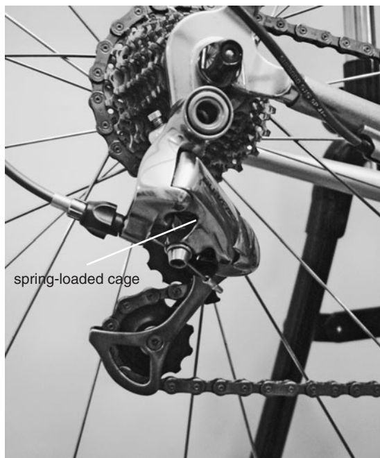
The spring-loaded cage on the rear derailleur is designed to keep tension on the chain as it moves between cogs on the rear cassette.
