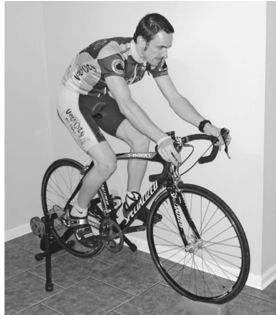
A stationary trainer locks the rear axle in place and provides resistance at the rear wheel.
