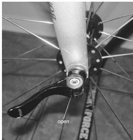
To release the wheel from the bike, open the skewer by pulling out on the skewer lever. (top shows the lever in the closed position; bottom shows the lever in the open position).
