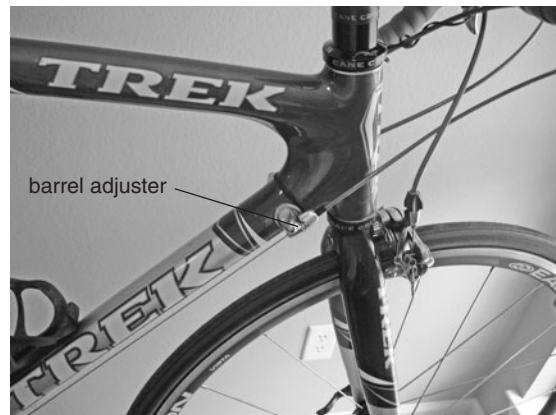
When riding, use the barrel adjusters on the down tube to make minor adjustments to shifting.
