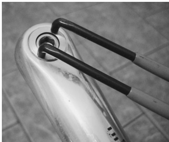
Use a pin spanner to remove the dust covers before reinstalling the crank arms.
