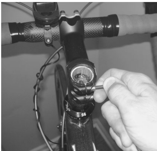
To remove the stem, remove the top cap and loosen the stem bolts.
