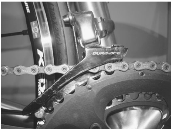
The front derailleur shifts the chain between chainrings on the crankset.
