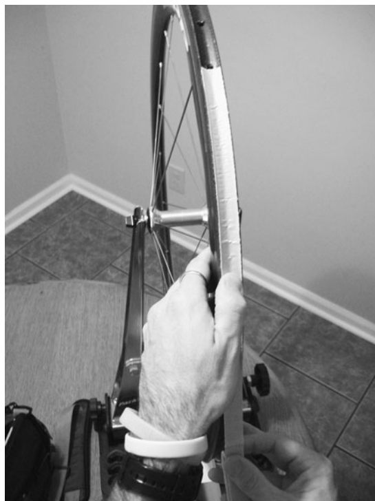
When applying a glue strip, make sure the rim is clean. A truing stand makes the job easier.
