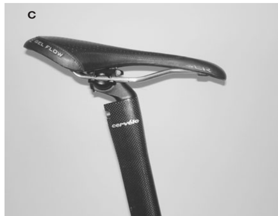
Various types of seat posts: in line (A), setback (B), and aero (C).
