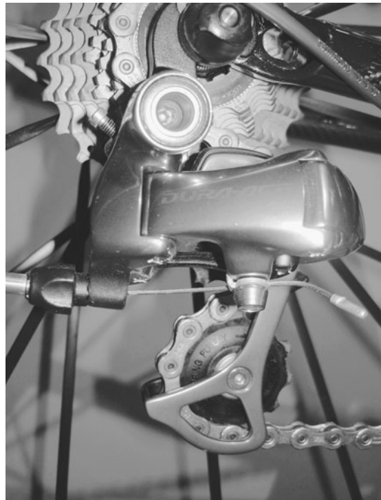
The rear derailleur shifts the chain between the cogs on the rear cassette.
