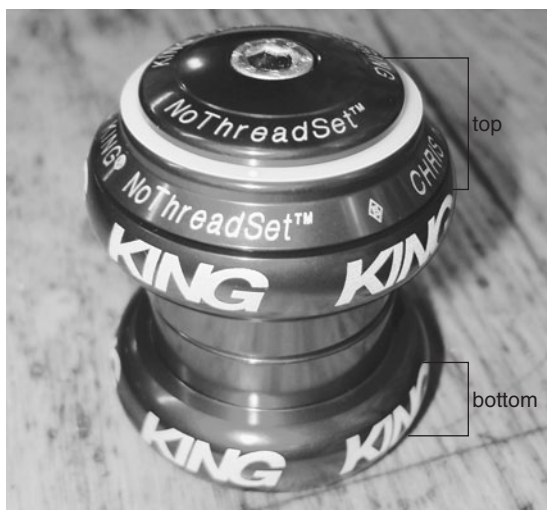
The headset is located at the top and bottom of the head tube and has bearings so the steerer tube can move smoothly.
