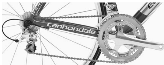
Gear combinations are determined by the number of teeth on the chainring and the number of teeth on the cassette.
