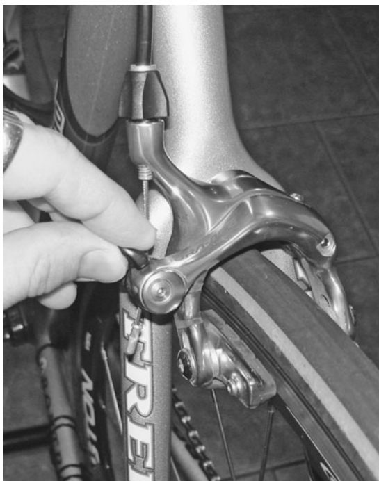
Lift the quick-release lever on the brake caliper to open the calipers and allow the wheel to slide free.
