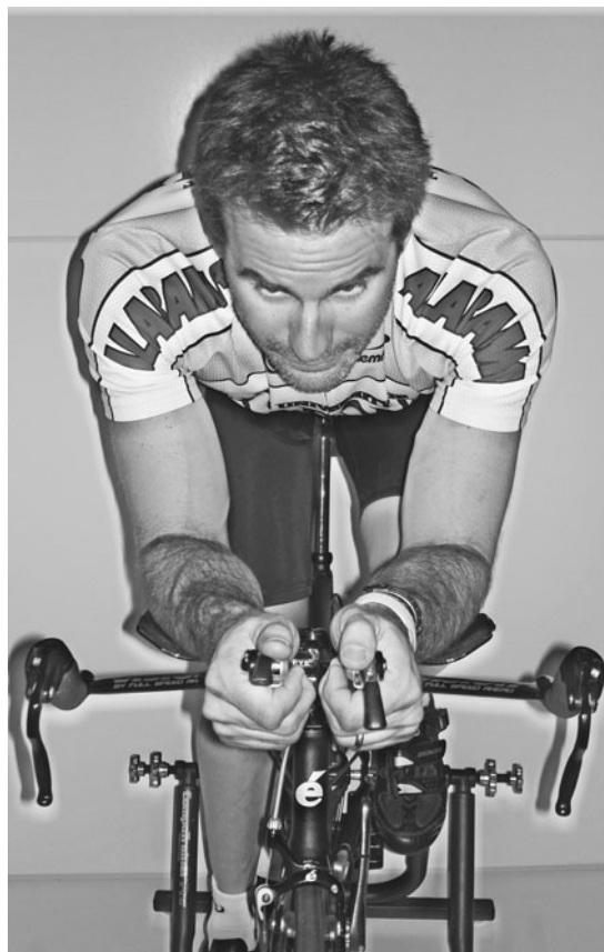
Position the aero bars as close together as comfort and safety allow.
