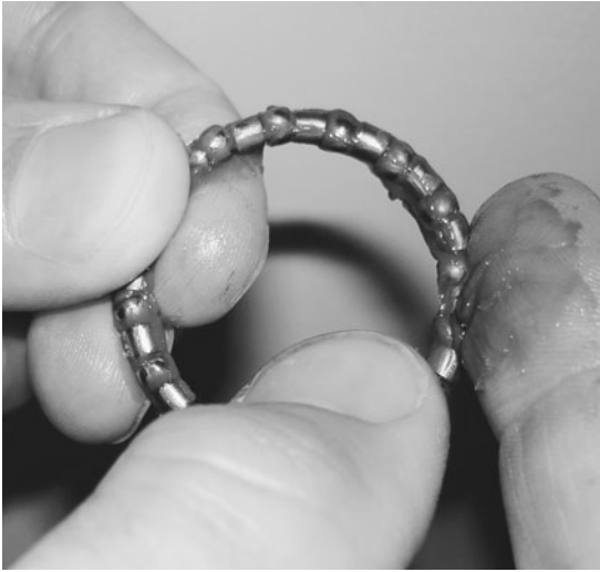
After cleaning the headset bearings, pack them with grease before replacing.
