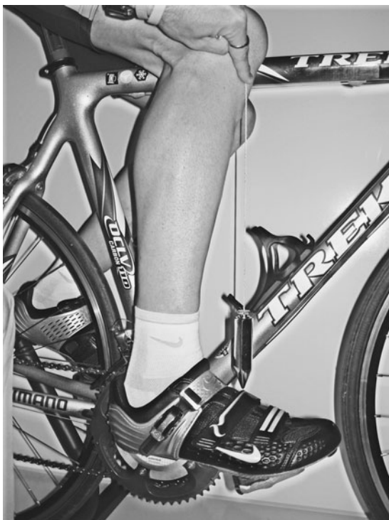
Use a plumb line to adjust the saddle's fore and aft position so the knee is aligned with the pedal axle.
