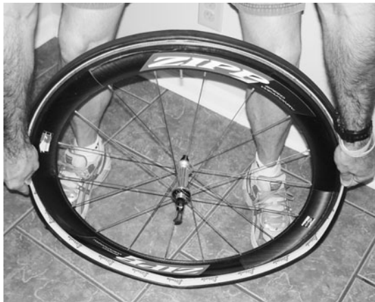
When placing the tubular tire back on the rim, start at the top and work your way to the bottom.
