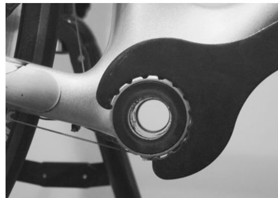
Bottom-bracket tools are specific to each type of bottom bracket. This is an outboard bearing bottom bracket.
