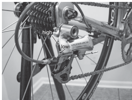
Adjusting the low- and high-gear limit screws on the rear derailleur prevents the chain from traveling into the spokes or becoming wedged between the cassette and the frame.
