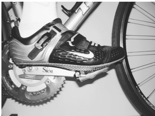
Clipless pedal systems provide a solid connection between the cyclist and the bike.
