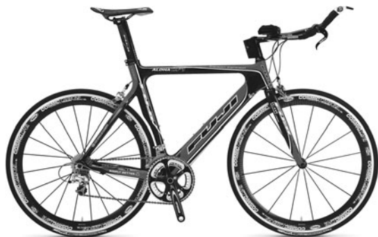
Time-trial bikes are designed to give an aerodynamic advantage when riding exposed to the wind, outside of a pace line. (Fuji)
