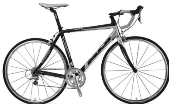
Compact-geometry frames differ from traditional frames in that they have a sloping top tube. (Fuji)
