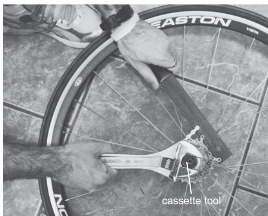
With one hand, hold the cassette in place with the chain whip. With the other hand, loosen the cassette lockring, using a large wrench placed on the cassette tool.
