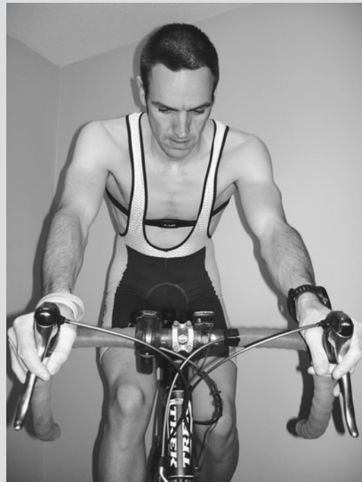
A heart-rate monitor consists of a transmitter, which is worn around the chest, and a display receiver, which is worn on the wrist or on the handlebars.
