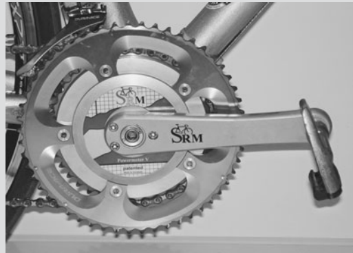
SRM cranksets are used to monitor power output while cycling.
