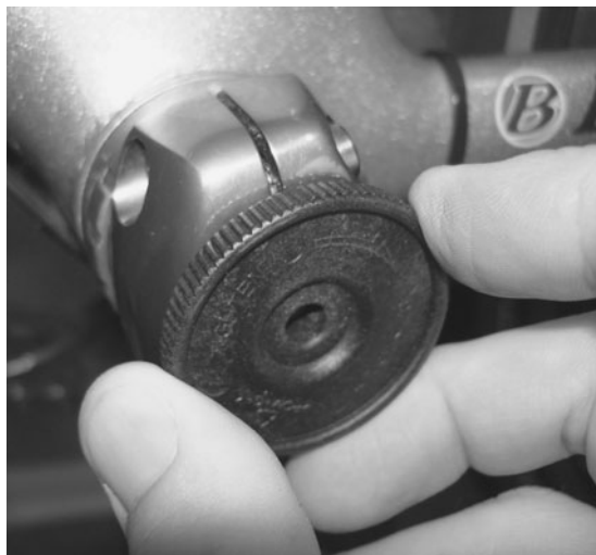
After loosening the crank-arm bolts, remove the crank-arm retention cap.
