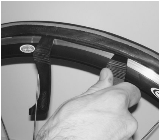
Tire levers are used to remove a tire from the rim by prying the tire bead up and over the rim wall.
