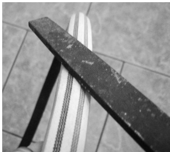
Inflating the tubular off the rim causes it to turn inside out, making it easy to abrade the base tape with a file.
