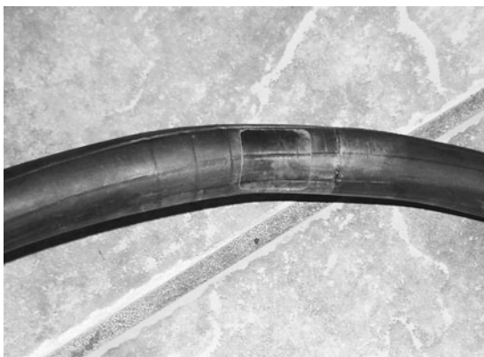
Once you find the hole in the tube, you can repair it with a glue patch or a self-adhesive patch.
