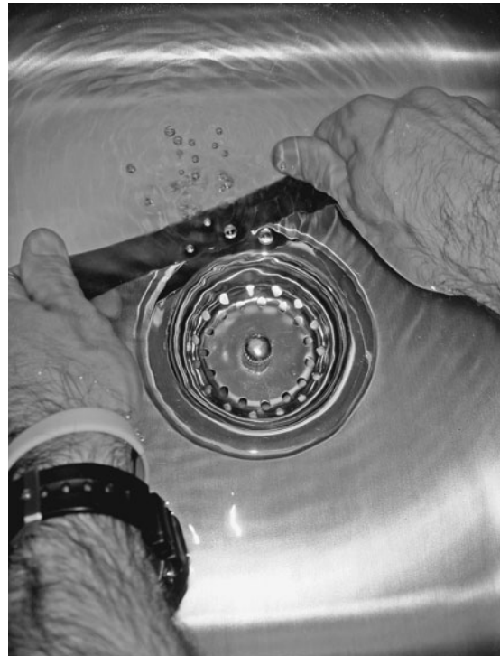
You can locate a small hole in an inner tube by inflating it, submerging the tube in water, and watching for bubbles.
