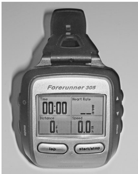
The Garmin Forerunner 305 functions as a cycle computer, a heart-rate monitor, and a GPS.
