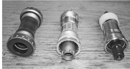
There are three basic styles of bottom brackets—from left to right: outboard bearing, cartridge-style splined, and cartridge-style tapered.
