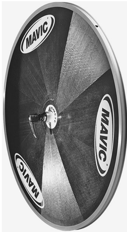
Aerodynamic race wheels are designed to cut through the wind, giving the rider an aerodynamic advantage. These wheels come with deep-dished rims (right) or as a full disc, which is used only as a rear wheel (left). (Mavic)
