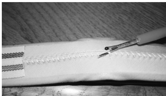
Once you locate the hole in the tube of a tubeless tire, use a seam cutter to cut the thread and open the casing.
