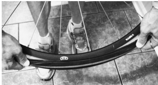
Once you replace the tube, work the tire back onto the rim. Be careful not to pinch the tube between the tire and the rim, and make sure the bead seats against the rim.
