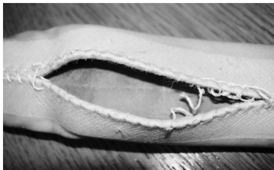
With the casing open, the tube is exposed and ready to be patched.
