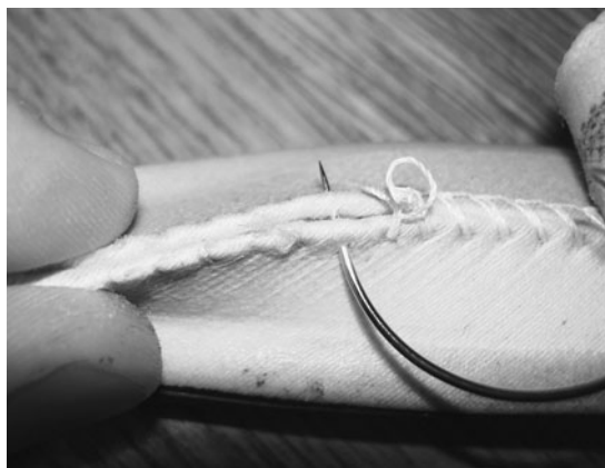
After patching the hole, sew the casing shut and glue the base tape back down.
