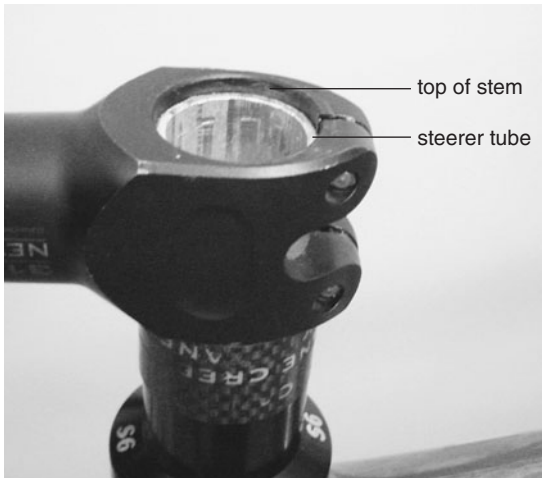
There should be a slight gap between the top of the stem and the top of the steerer tube.
