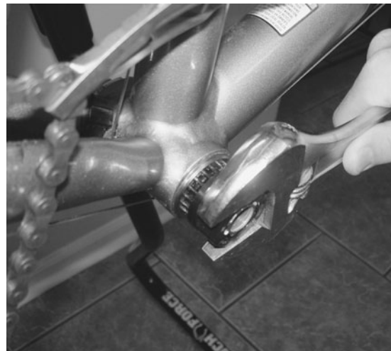
With a cartridge-style bottom bracket, remove the bottom bracket by loosening and removing the right side first.
