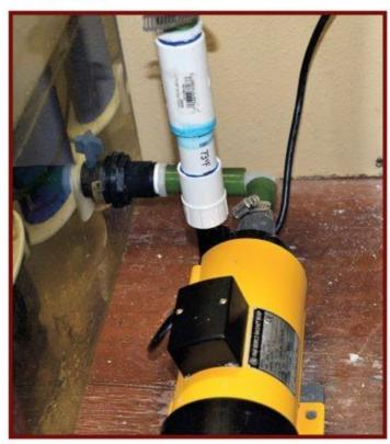
To minimize heat transfer to the aquarium water, an external pump was chosen over a submersible type.
