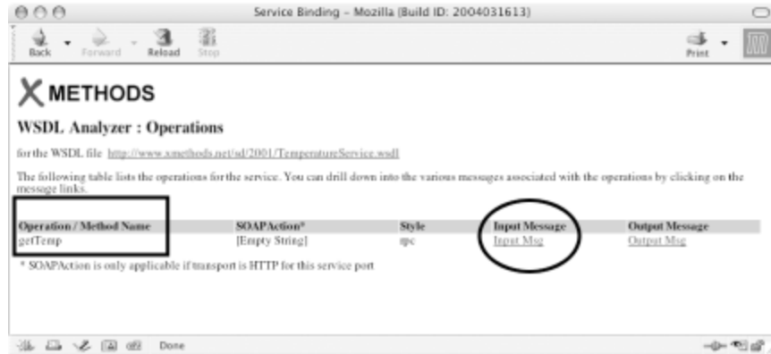
Figure 8-4. The description of the single operation that is part of the weather-temperature service
