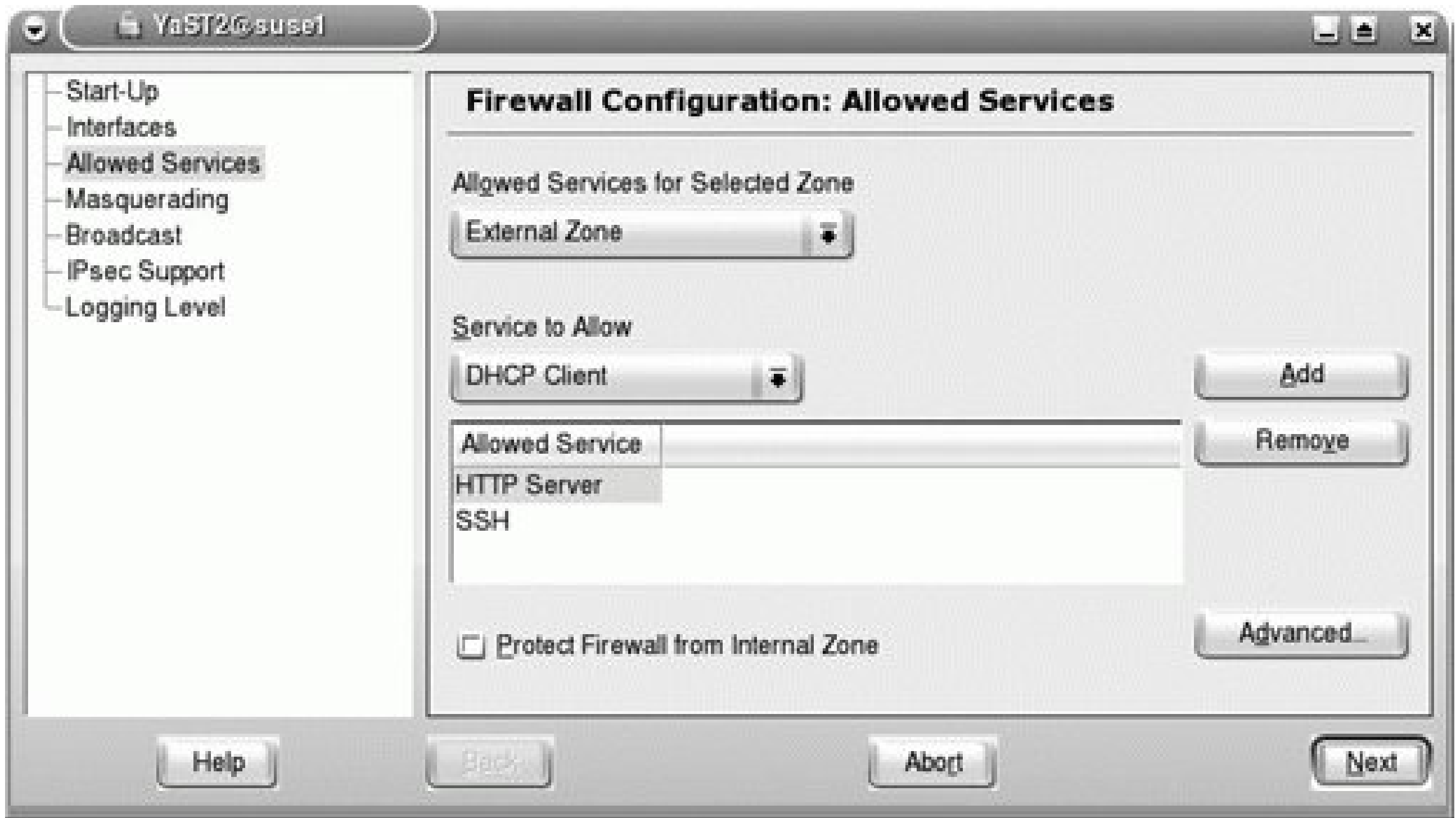
Figure 8-6. Customizing a firewall in SUSE YaST
