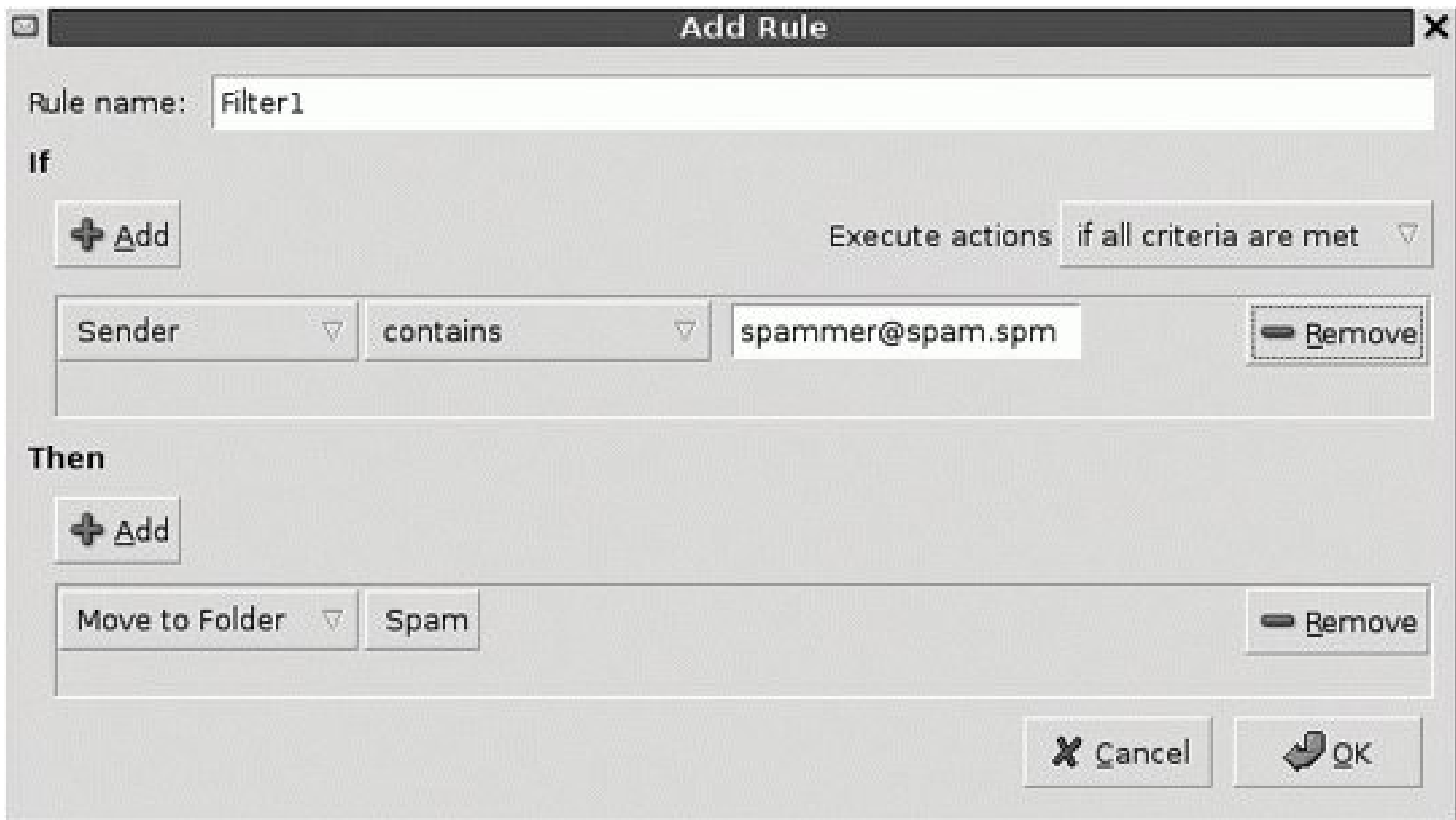
Figure 3-3. Adding a spam filter rule
