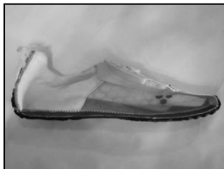
Terra Plana VivoBarefoot Evo cut in half. Note the heel and forefoot are the same height. Both are good qualities in minimalist shoes.
