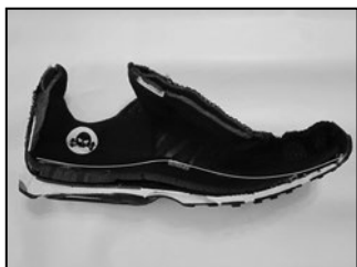
Typical running shoe cut in half. Note the extreme difference between thickness of heel and forefoot. Also note high arch support. Neither is good.
