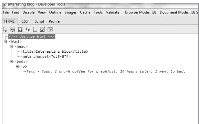
FIGURE 1.3 Internet Explorer 8, like all other browsers, adds missing elements in the DOM. (IE seems to swap <title> and <meta> , however.)
