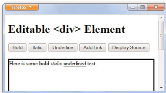
FIGURE 5.4 Underlined text in the editdiv.html example.
