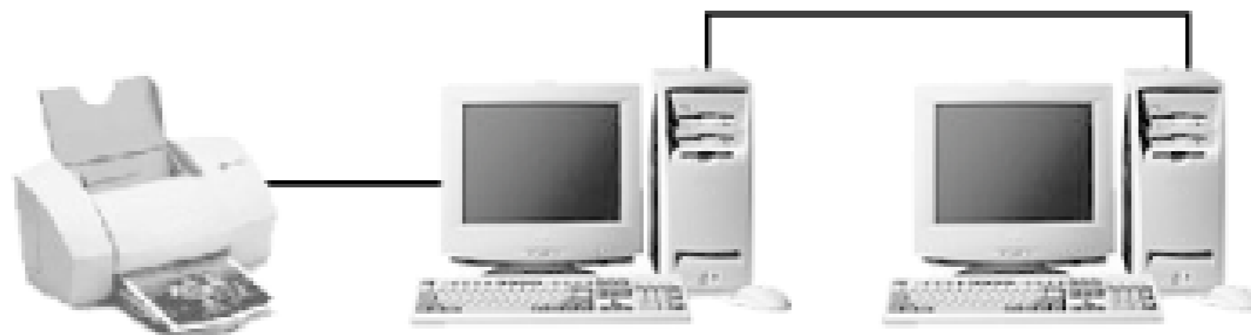
Figure 7-2. A quick-and-dirty hubless workgroup; given its limitations, however, it's best suited as a temporary solution
