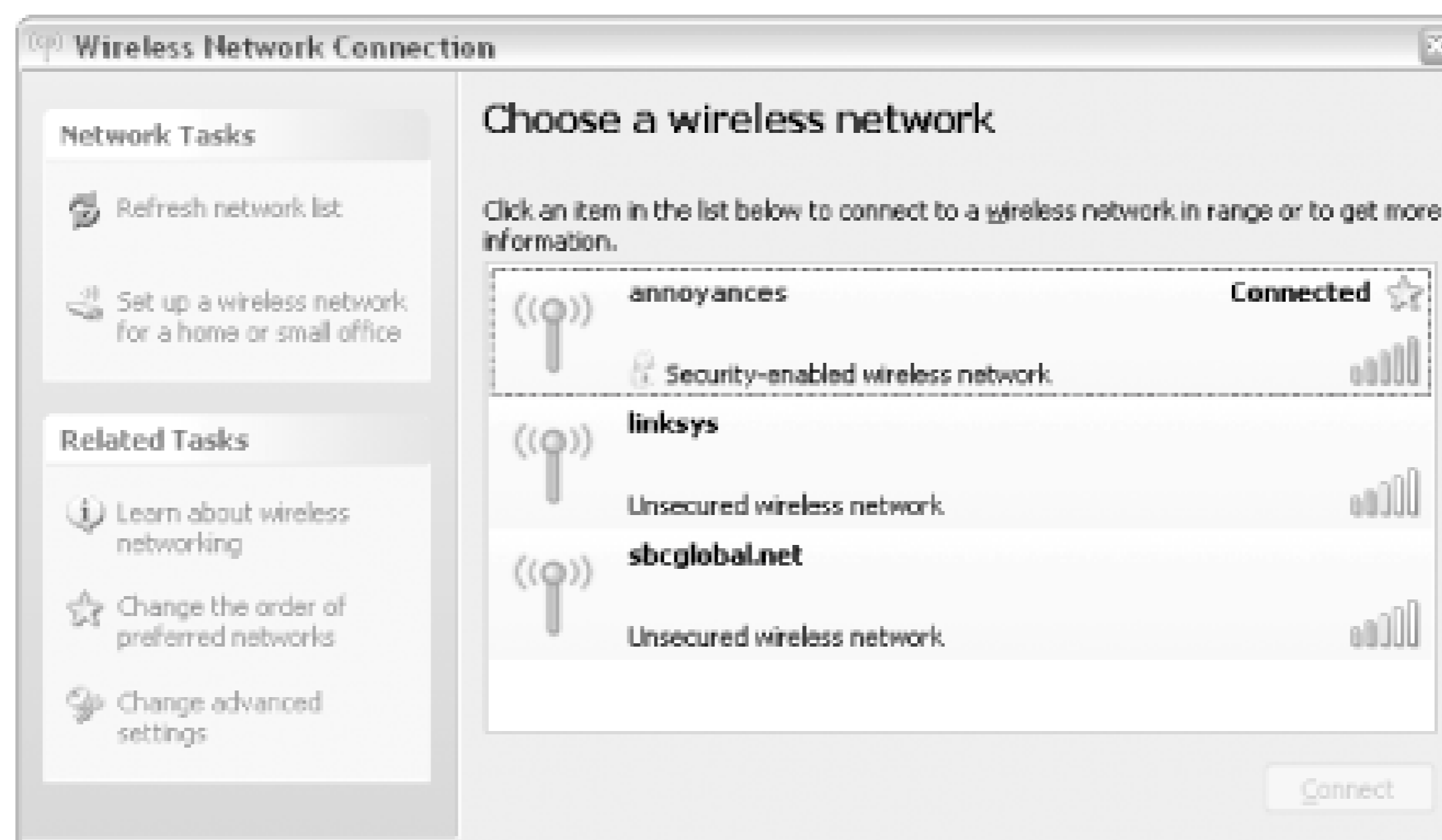
Figure 7-20. The WiFi sniffer in Windows XP SP2 lets you connect to any available WiFi network
