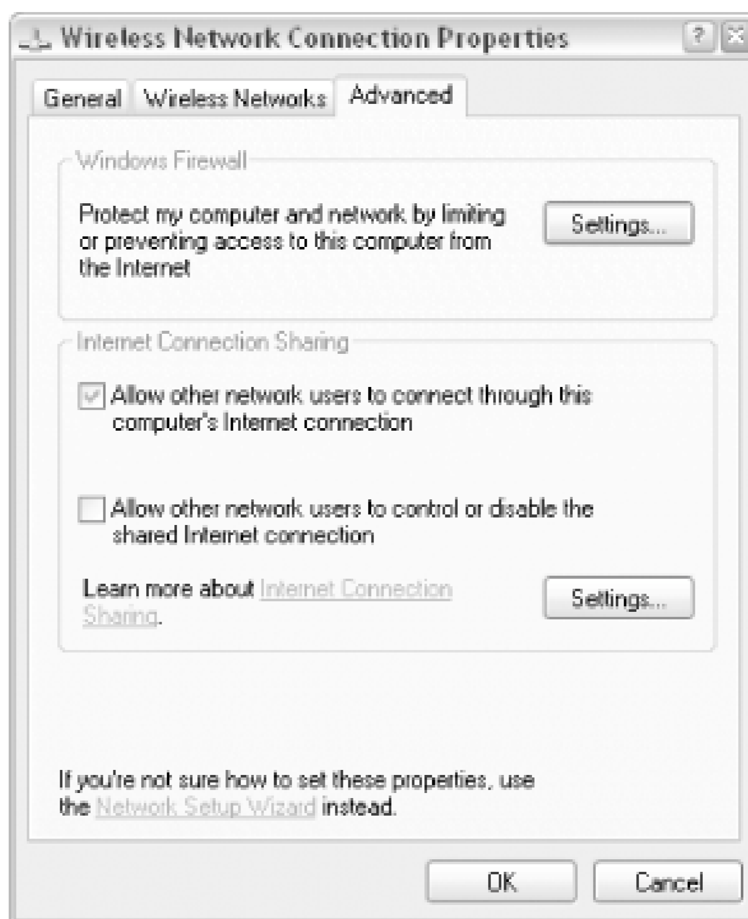
Figure 7-12. Any Internet connection can be shared with other computers in your workgroup
