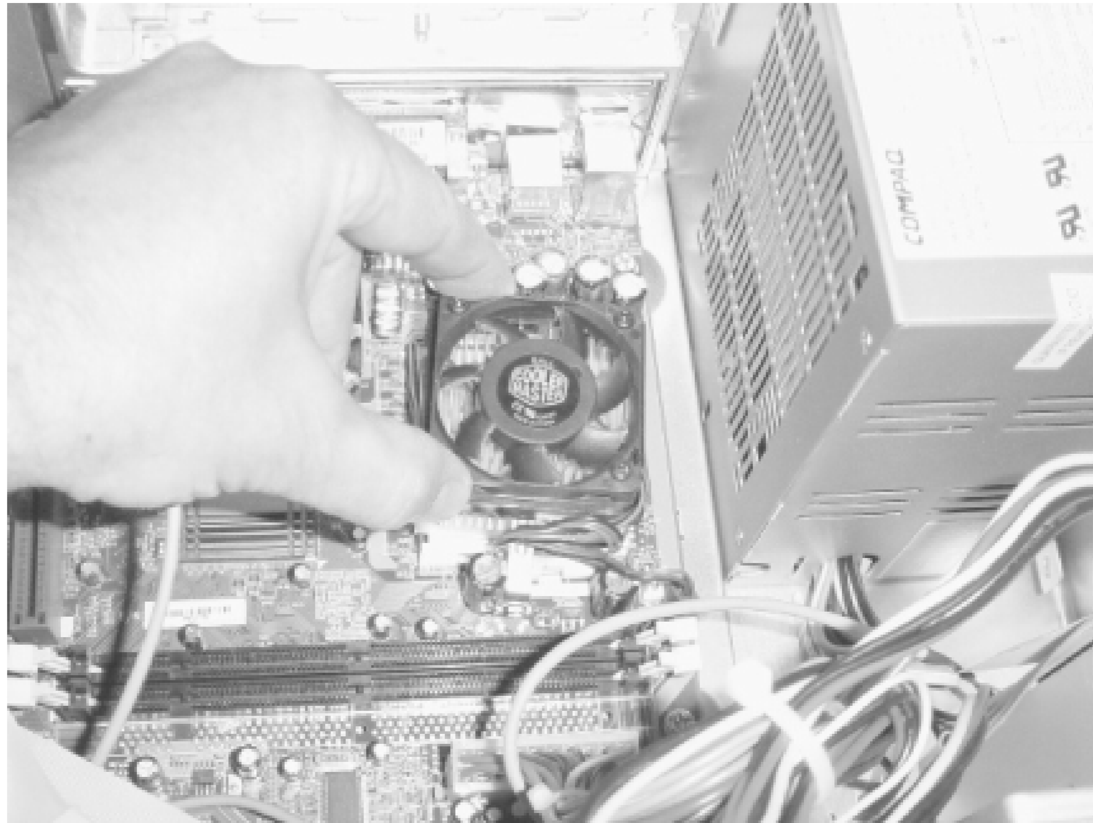
Figure 3-20. Slight pressure and twisting bonds the heat sink to the CPU
