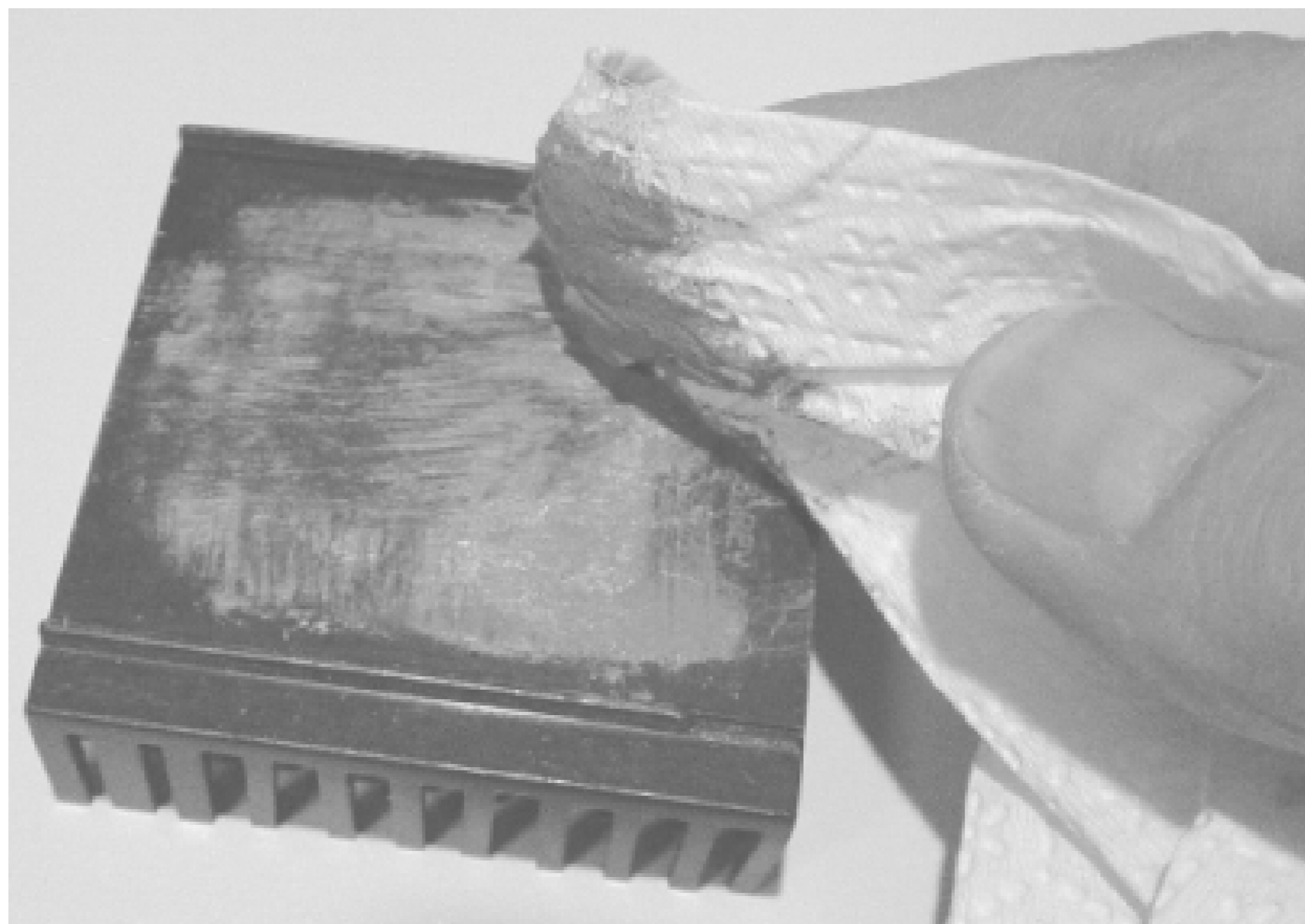
Figure 3-17. Wiping excess compound from heat-sink surface
