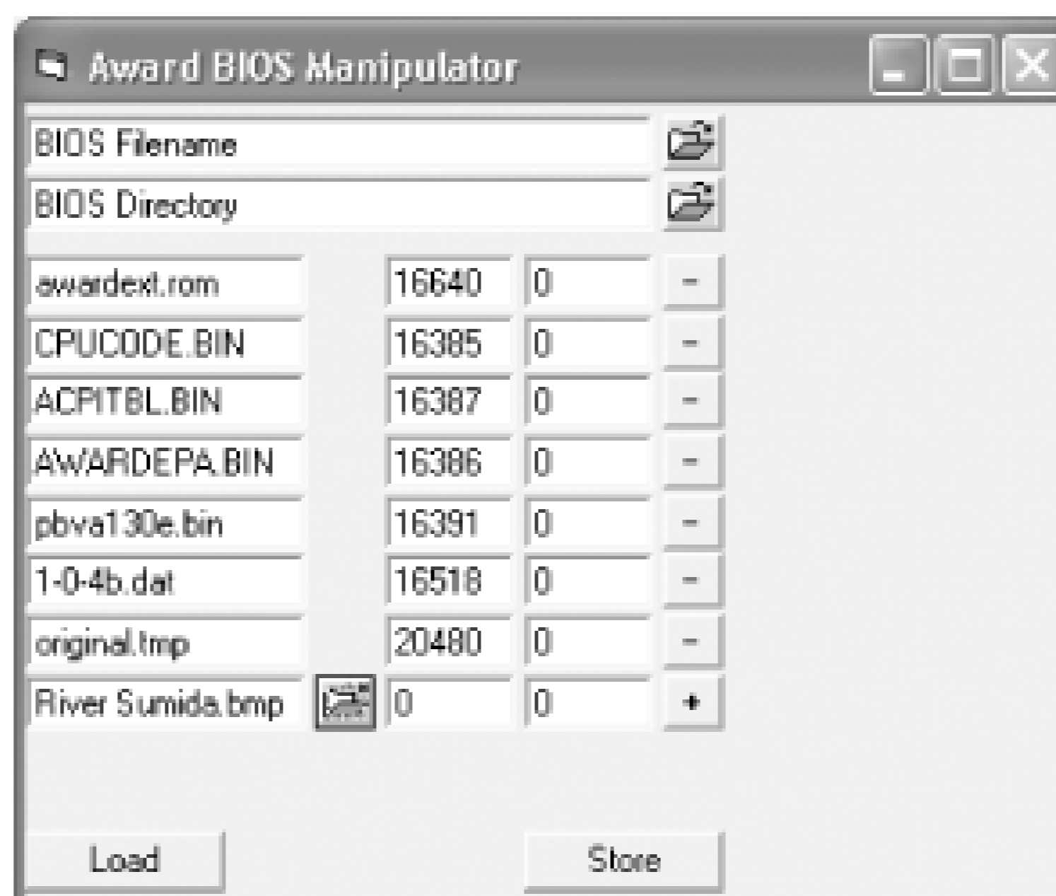
Figure 1-7. The AwardMod program lets you see which feature modules are in your BIOS and add your logo
