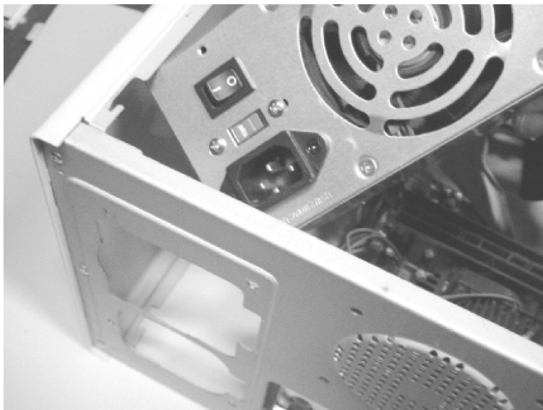
Figure 3-6. Removing the power supply from the chassis
