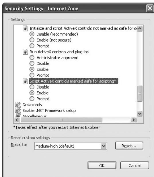
Figure 1-3 The property window used to change the security settings in Internet Explorer
