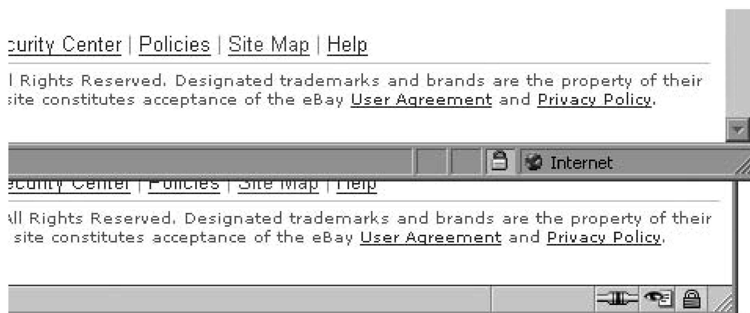
Figure 3-6. The little padlocks at the bottom of your browser window (both Internet Explorer and Mozilla shown here) tell you that you are using a secure connection
