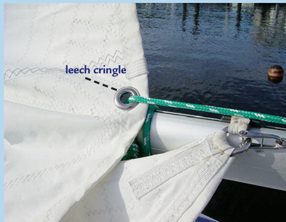
B. Tighten leech line to stretch foot of sail along boom
