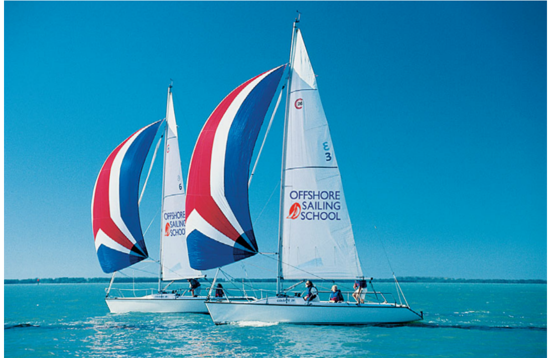
Figure 9-5. Both spinnakers are properly set: tack and clew are level.
