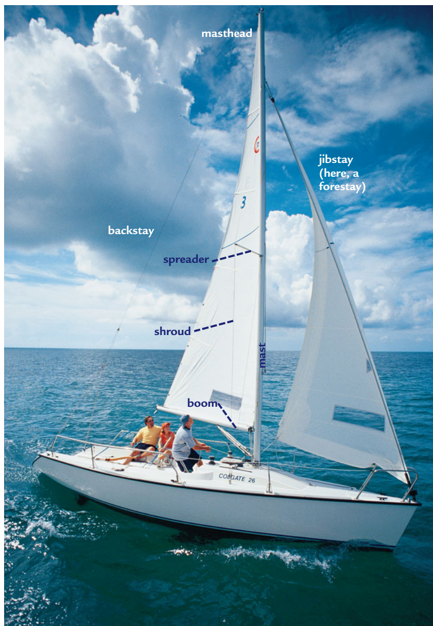
Figure 1-3. Terms that describe standing rigging.
