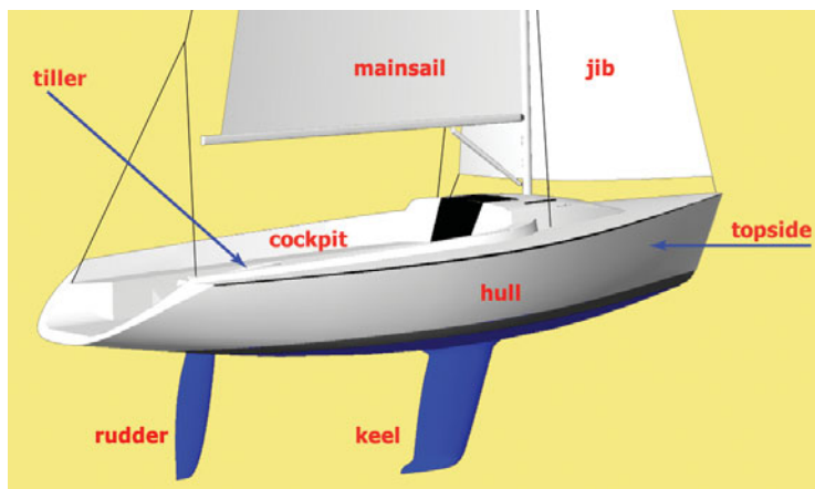
Figure 1-2. Terms that describe the parts of a sailboat.
