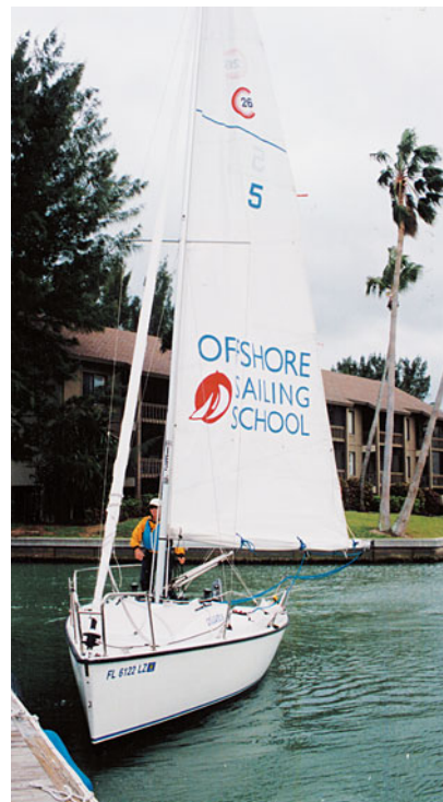
Figure 7-4C. Turning alongside. Back mainsail if necessary to kill speed.
