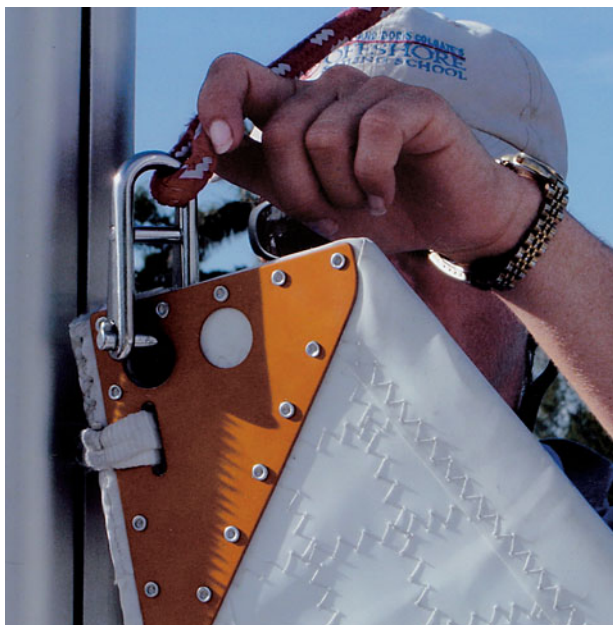
Figure 2-3. Attaching halyard to the head of the sail.
