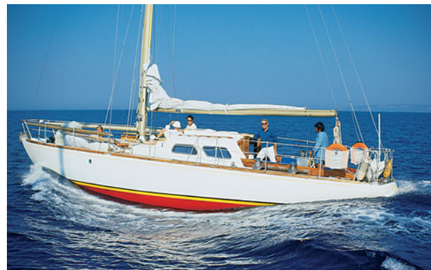
Right: Hull speed is shown in one long wave between the bow and stern.
