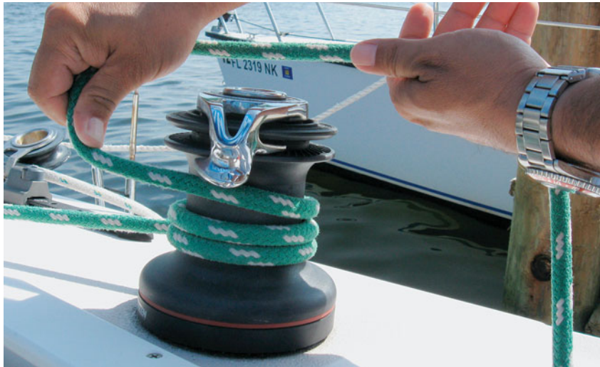
Figure 10-2. The proper way to put wraps around a winch.
