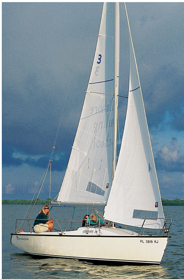
Figure 2-5. Backing the jib to get underway.
