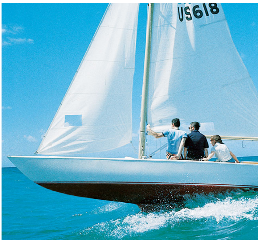
Figure 5-10. When sailboats surf, hull speed is exceeded.
