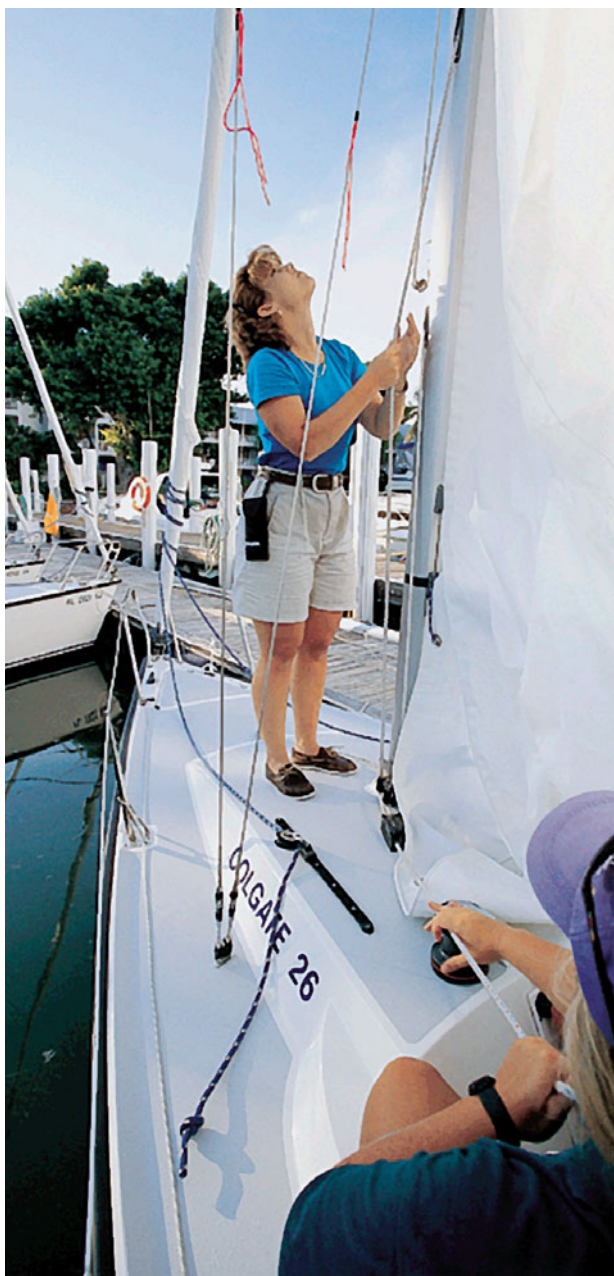
Figure 1-5. Raising a sail with the halyard (running rigging).
