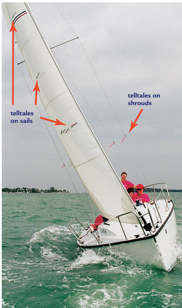
Figure 4-5. Telltales on the sail help you see airflow. Telltales on the shrouds help you see wind direction.
