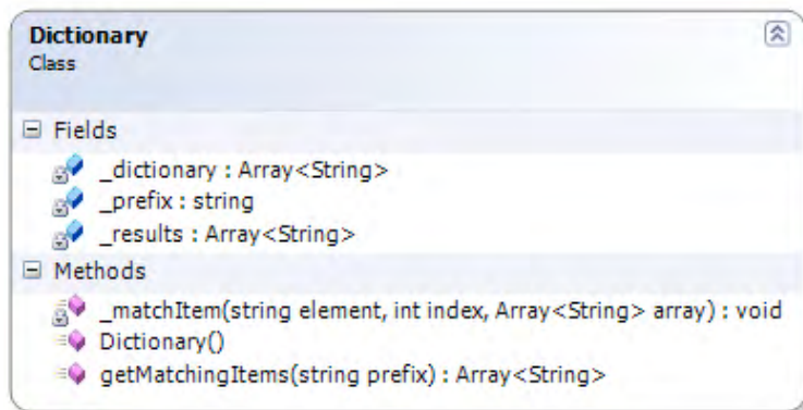
Figure 7-3. Diagram representing the Dictionary class
