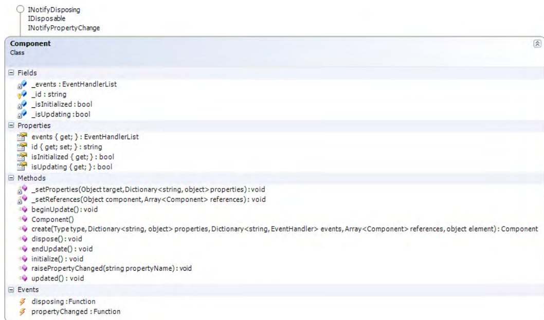
Figure 6-1. Class diagram for Sys.Component
