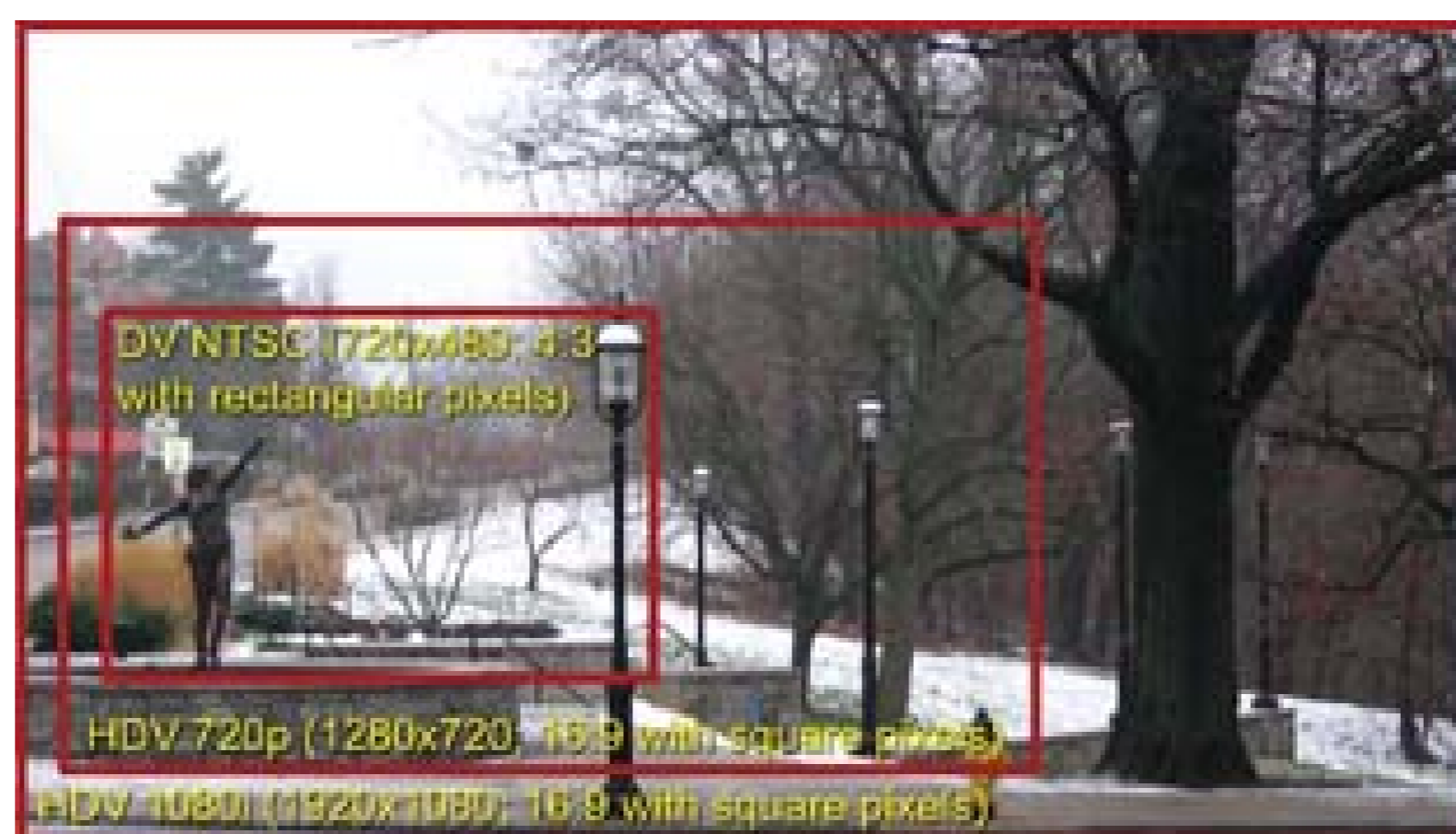
Figure 3-24. Relative resolutions for DV, HDV 720p, and HDV 1080i
