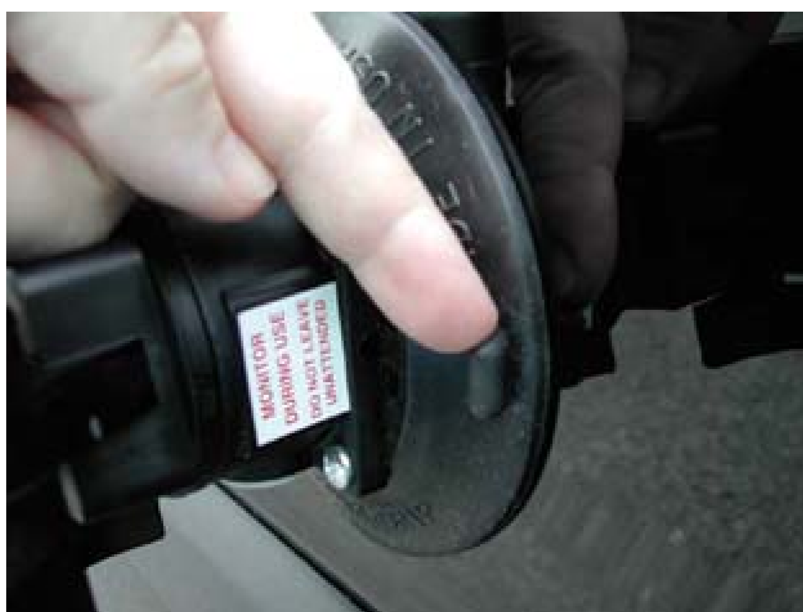
Figure 3-6. Pull on the tab firmly to release the vacuum
