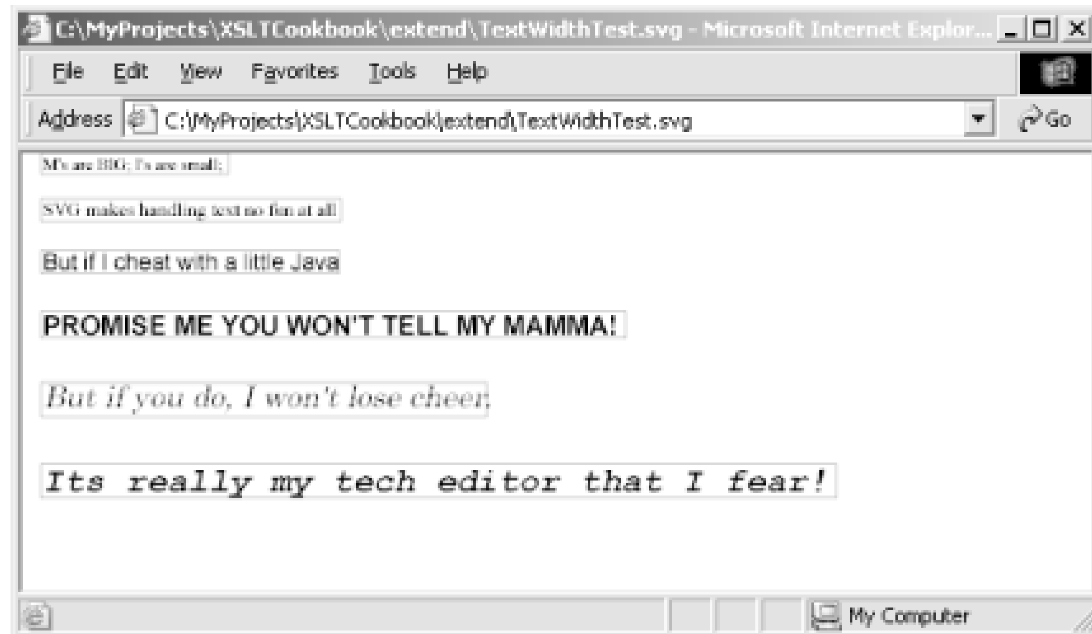
Figure 12-1. Creating correctly sized text-bounding rectangles with the SVGFontMetrics extension
