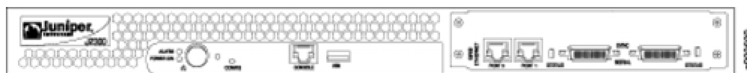
Figure 2-12. J2300 dual FE/serial ports with right-to-left numbering
