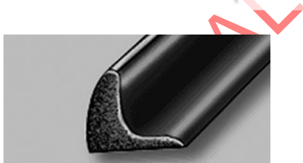
Figure 5.9 General Motors type "K" trunk rubber—close view.
