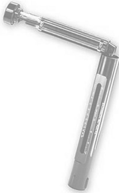
Figure 7.2 A typical sling psychrometer.
