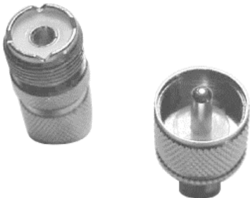
Figure 6-15. The so-called "UHF" connector
