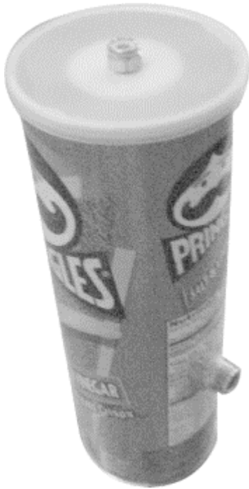
Figure 7-3. The completed antenna
