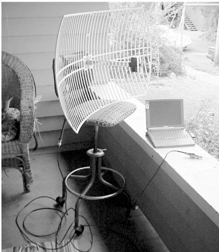
Figure 6-11. A 24dB parabolic dish
