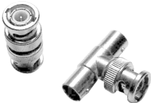
Figure 6-12. BNC: Bayonet Navy Connector (or Bayonet Neill Concelman, depending on who you ask)
