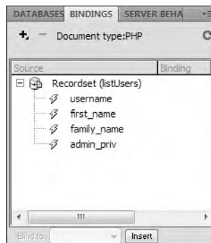
Figure 14-13. The Bindings panel gives access to the query result.
