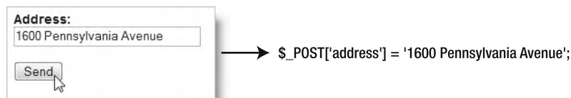
Figure 11-2. The $_POST array automatically creates variables with the same name and value as each form field.
