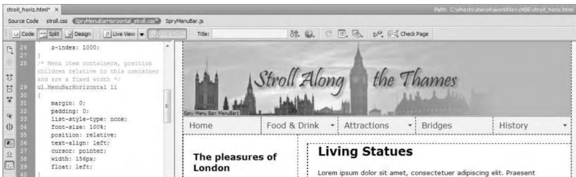
Figure 6-13. Giving the <li> elements a fixed pixel width matches the width of the container <div>.
