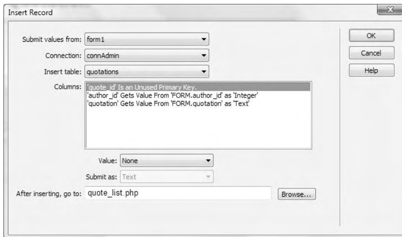
Figure 16-12. The Insert Record dialog box matches form fields with table columns.
