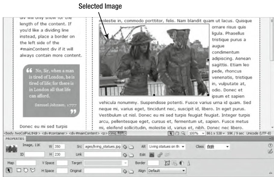
Figure 1-19. The Property inspector gives access to the main attributes of the <img> tag when an image is selected.
