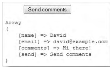
Figure 9-7. The PHP $_POST superglobal array contains the data submitted from the form.
