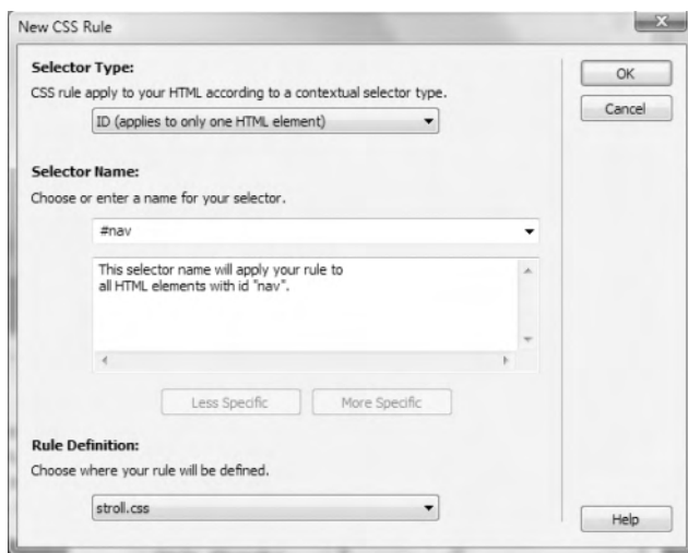
Figure 6-9. The settings for creating the style rule for the nav <div>
