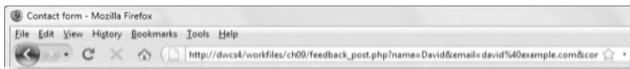
Figure 9-8. Data sent using the GET method is appended to the URL as a series of name/value pairs.
