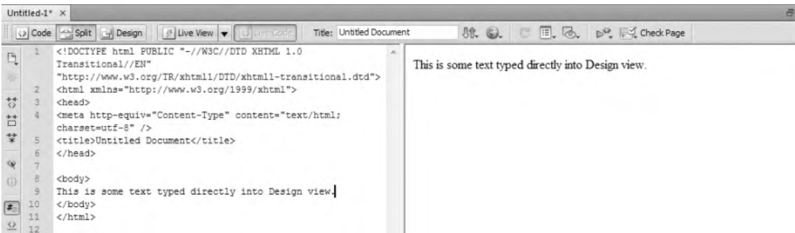
Figure 3-4. Anything entered in Design view is replicated in Code view.
