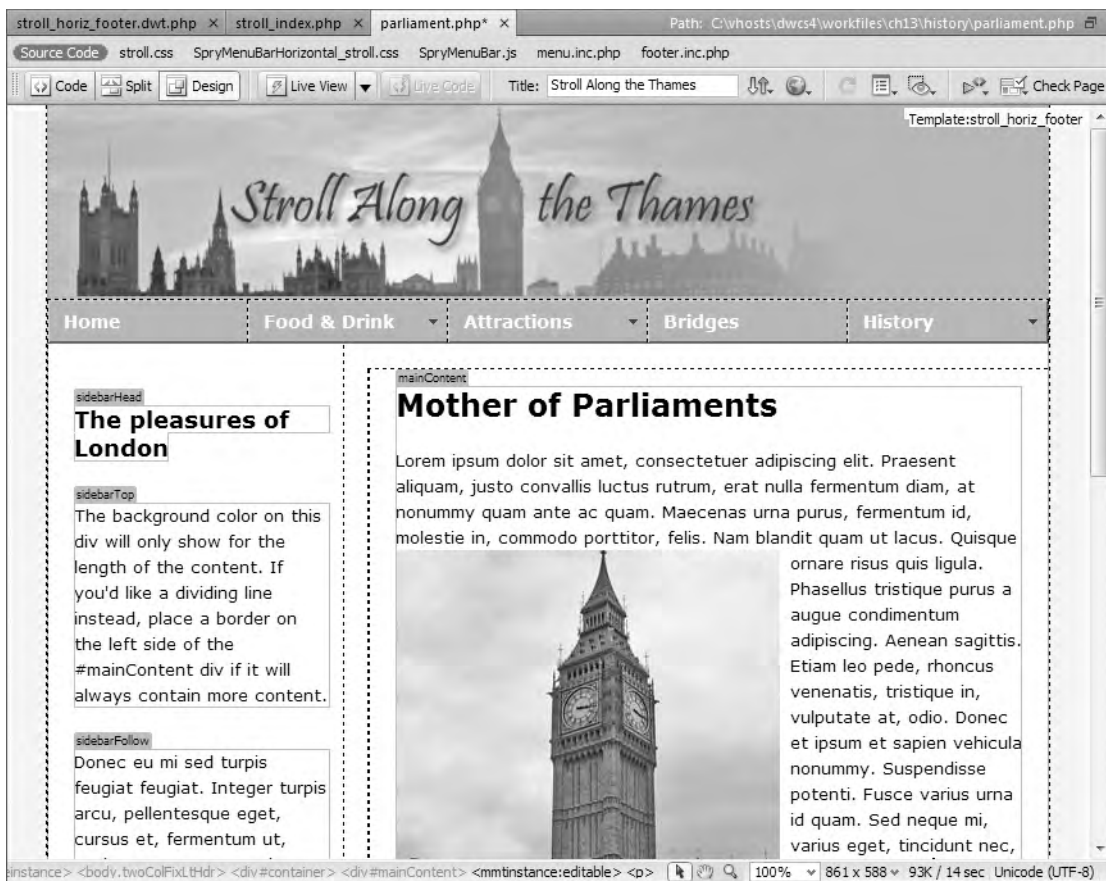
Figure 13-8. The optional region has been removed from the sidebar.
