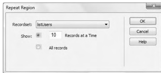
Figure 14-14. A repeat region can display a selected number of records or all of them.
