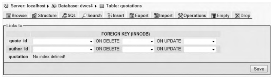
Figure 16-7. Relation view lets you specify what happens when a record in a parent table is deleted or updated.
