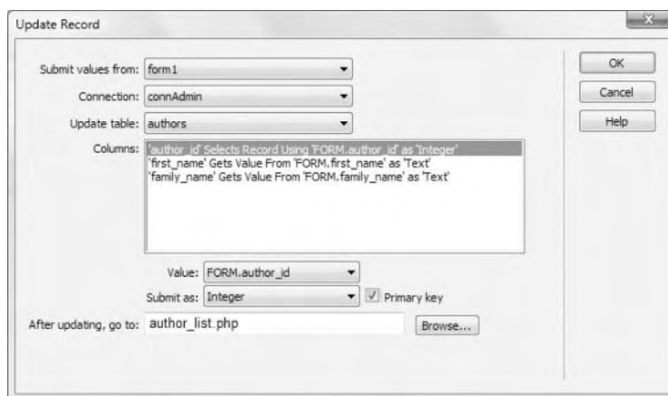
Figure 16-14. The Update Record dialog box uses the primary key to identify the record being updated.
