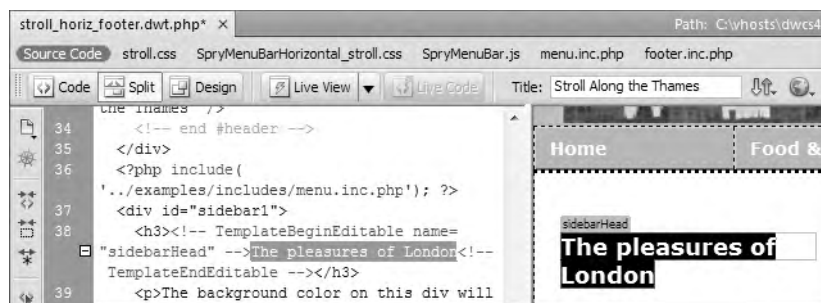
Figure 13-1. Editable regions are easily identified in both Code view and Design view.
