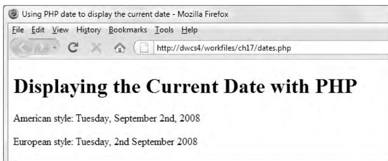
Figure 17-21. The PHP date() function formats the current date or a Unix timestamp in various styles.
