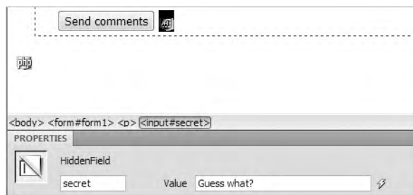
Figure 9-9. Select a hidden field's icon in Design view to edit its name and value in the Property inspector.
