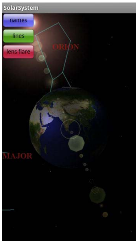
Figure 8–11. Putting UI components on top of an OpenGL screen
