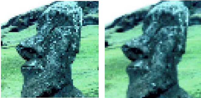
Figure 5–20. The left side has all filtering turned off. The right side has bilinear filtering turned on.
