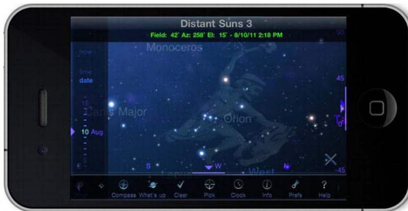
Figure 8–12. Distant Suns with custom date wheel on the left side yet with a standard UIKit toolbar at the same time
