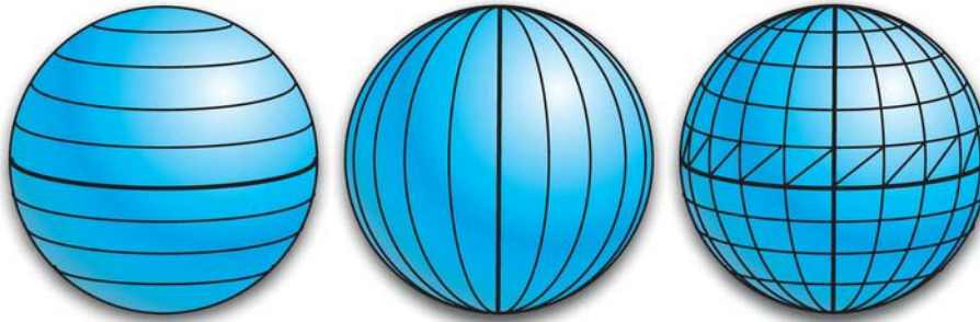
Figure 3–15. Stacks go up and down, slices go round and round, and faces are subdivided into triangle strips.
