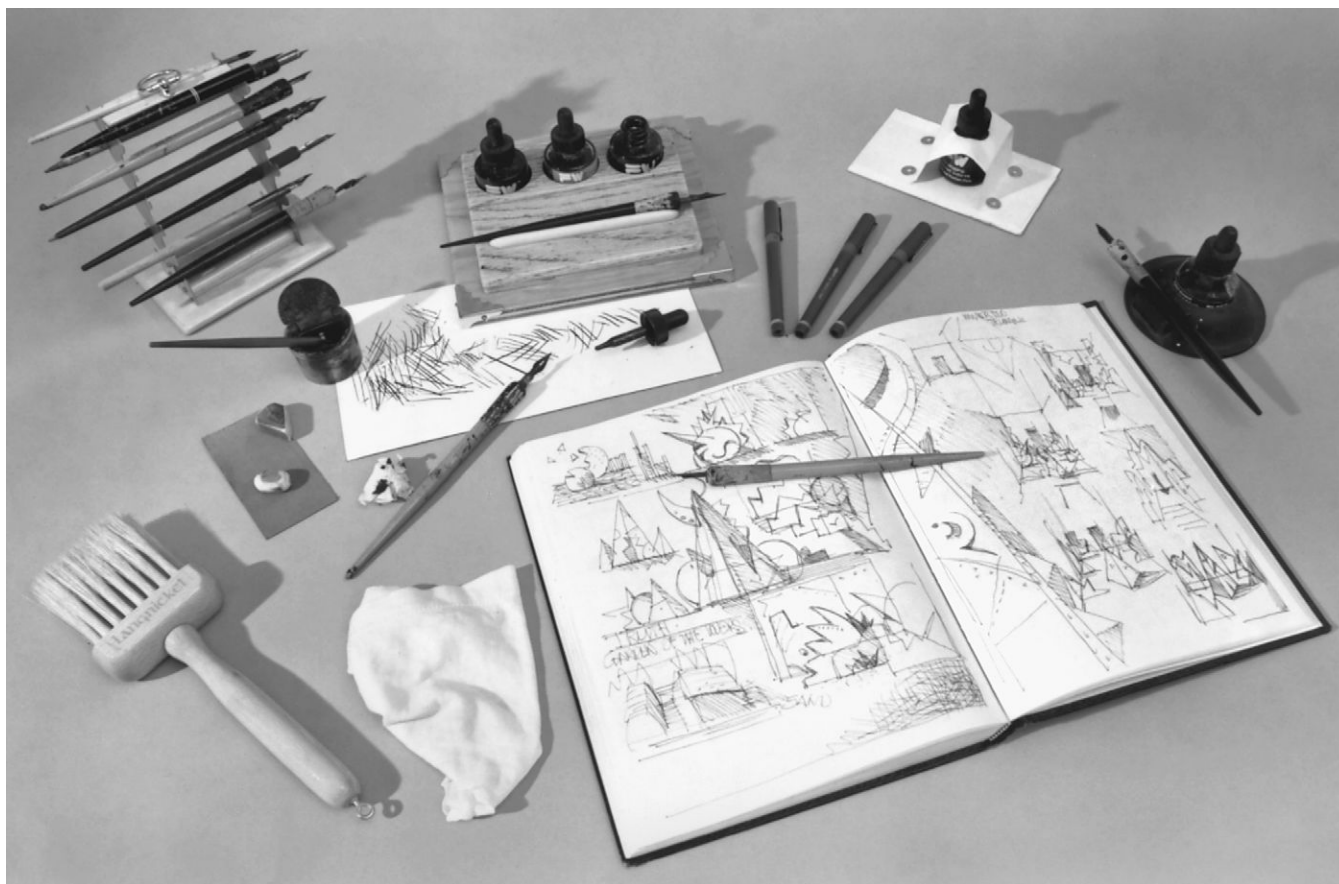
FIGURE 4-13 Setting up for ink drawing. Clockwise from top left: holder for steel quill pens; metal school inkwell; wood holder for ink bottles and paper for testing pens; technical pens; cardboard holder for inkwell; rubber Higgins ink bottle holder; sketchbook with #99 Hunt drawing point; soft cloth for wiping pens; brush; #512 Hunt extra-fine bowl; tissue; Sanford MagicRub erasers. (Photo: Kathryn Drinkhouse)
