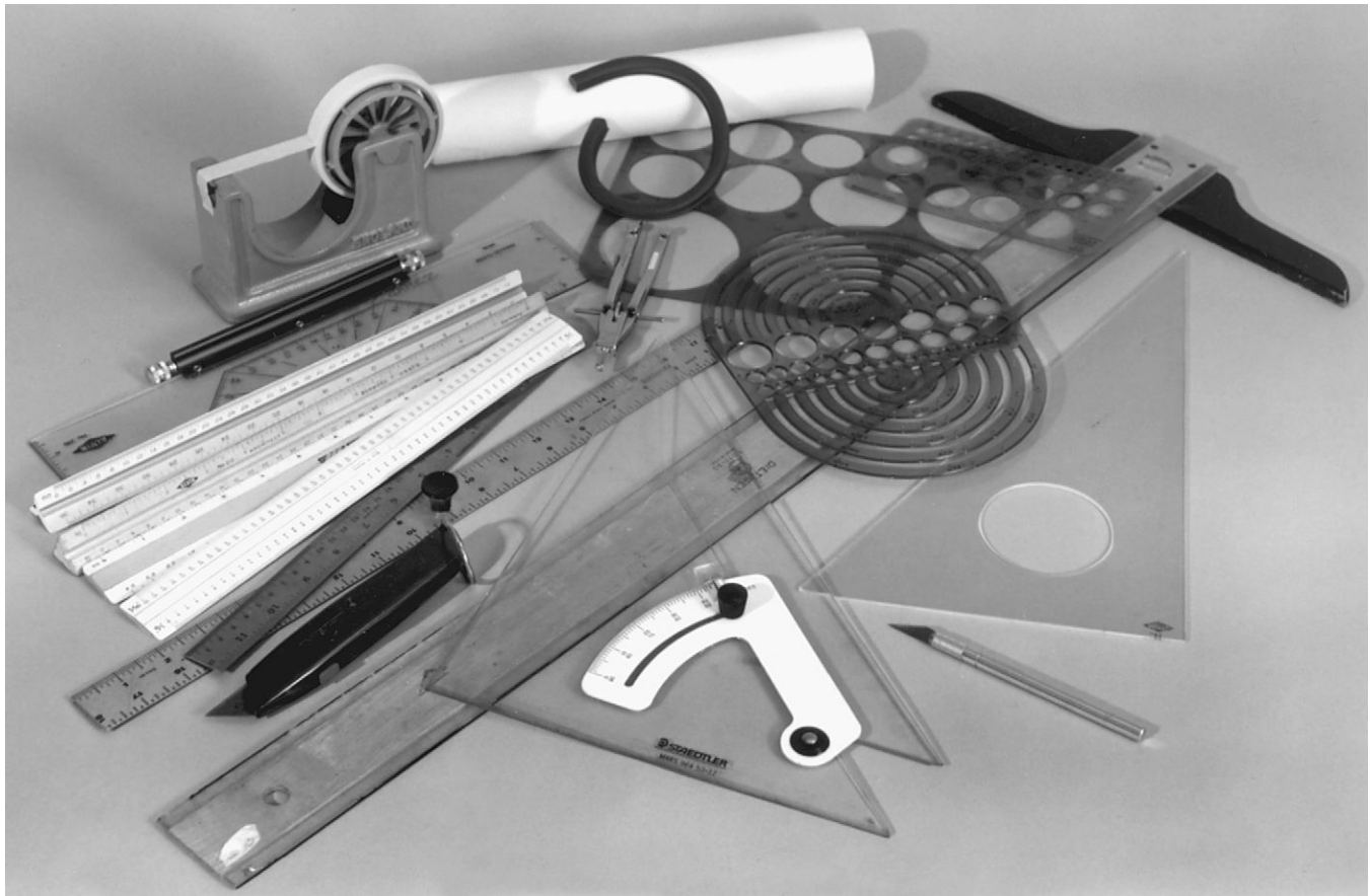
FIGURE 4-2 Clockwise from top left: drafting-tape dispenser; tracing paper; flexi-curve; circle templates; T-square; clear plastic triangles; X-Acto knife; adjustable triangle; heavy-duty mat knife; metal straightedge; compass; architects' and engineers' scales; a parallel glider. (Photo: Kathryn Drinkhouse)
