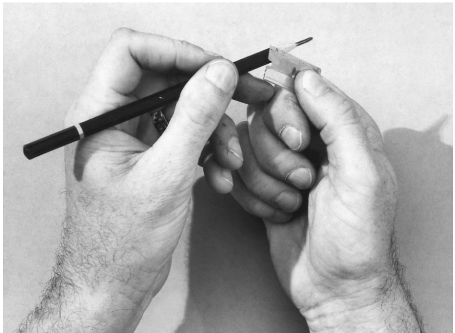
FIGURE 4-6 To sharpen the pencil, cut back the wood to a long taper, exposing about a quarter-inch of lead. (Photo: Kathryn Drinkhouse)
