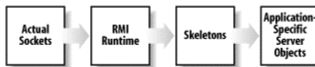
Figure 8-1. Runtime structure for RMI servers
