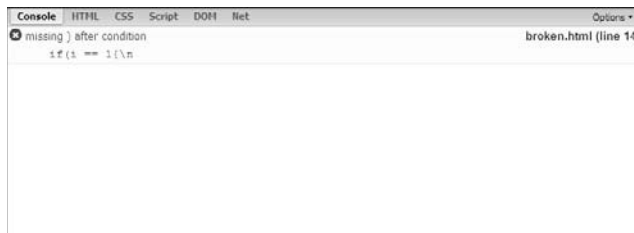
Figure 4-9: The Firebug tool shows an error. Click the error line to see it in context.
