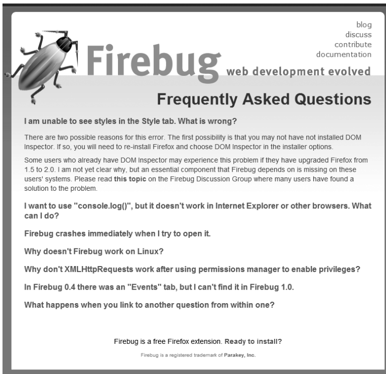
Figure 8-3. FAQ using :target shows the question you clicked in the open position.
