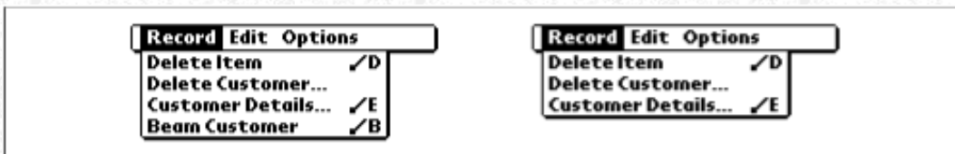
Figure 3- 17. The Record menu with beam present and not present
