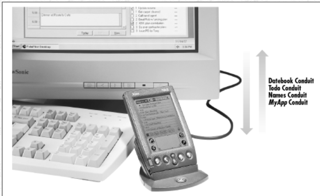
Figure 2- 1. Conduits control the exchange of information
