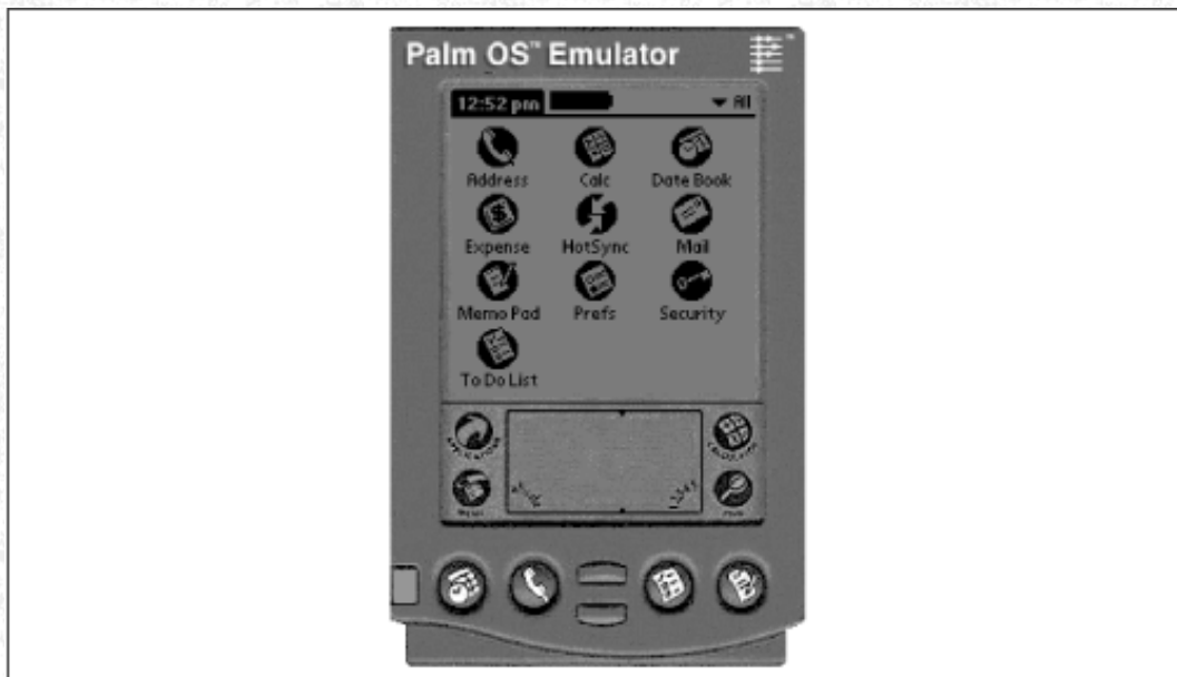
Figure 2- 6. POSE in a desktop window emulating a Palm III device
