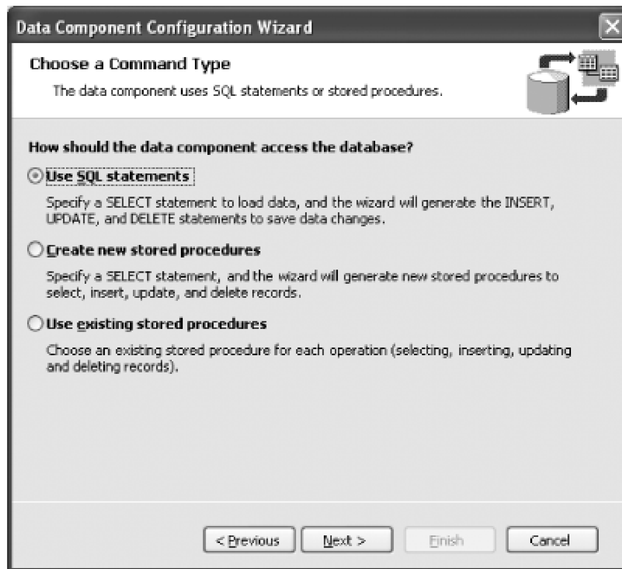
Figure 4-56. Selecting how the data component will access the database
