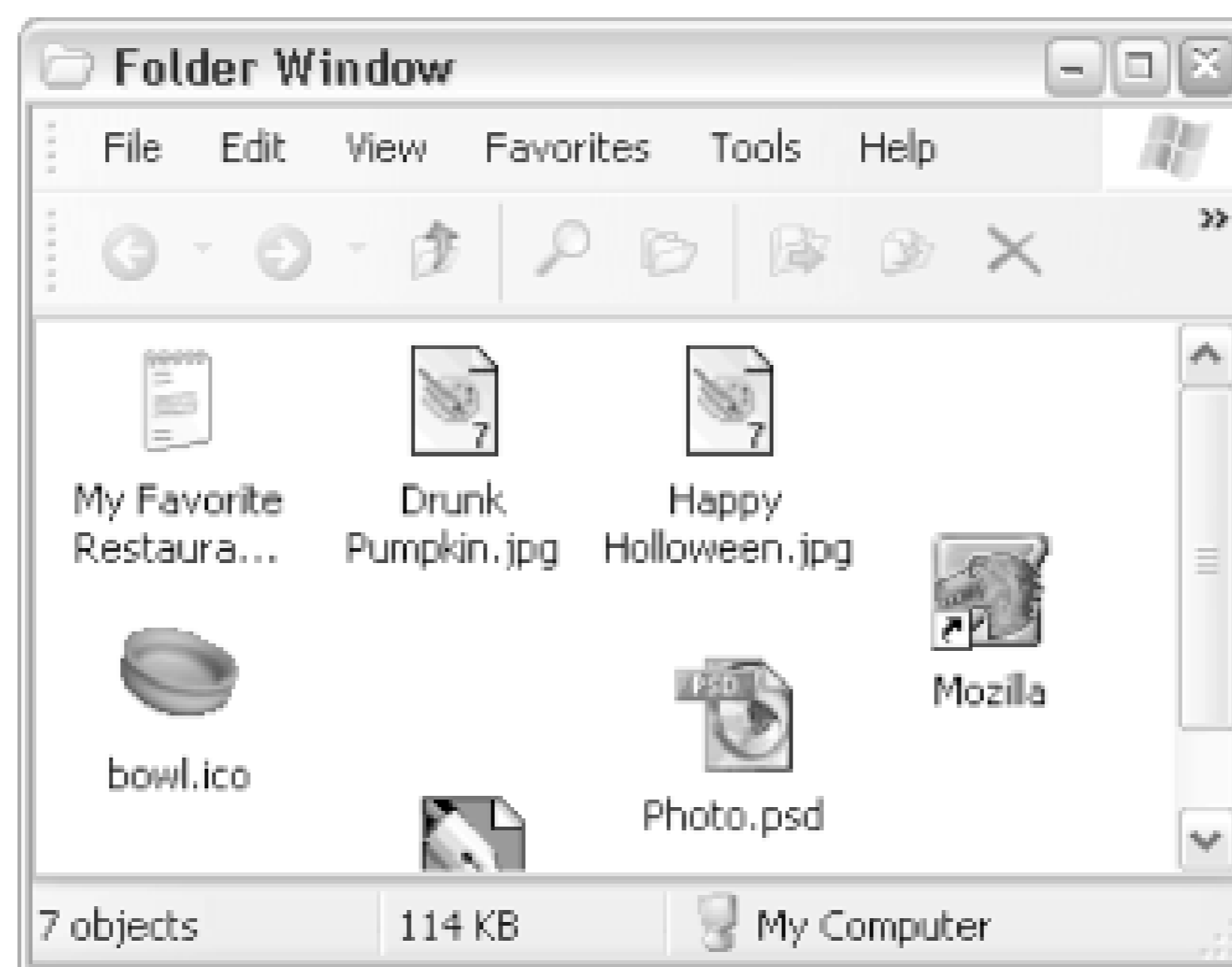
Figure 1-2. Windows are typically decorated with a title bar, title buttons, a menu bar, and a scrollable client area
