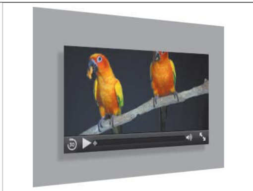
FIGURE 7.14 The video and background div are rotated at a 40-degree angle around the Y axis in Safari 5.1.
