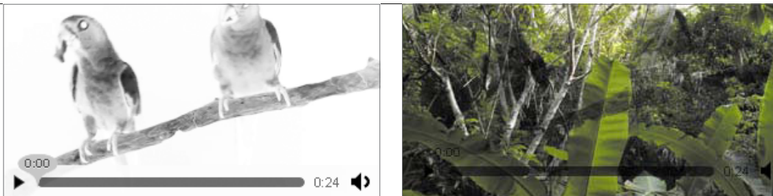
FIGURE 10.13 The video with the luminanceToAlpha colour matrix type applied to it (left). The large white areas are transparent, and a background image would show through them, as shown on the right, where you can barely make out the parrots and the branch.
