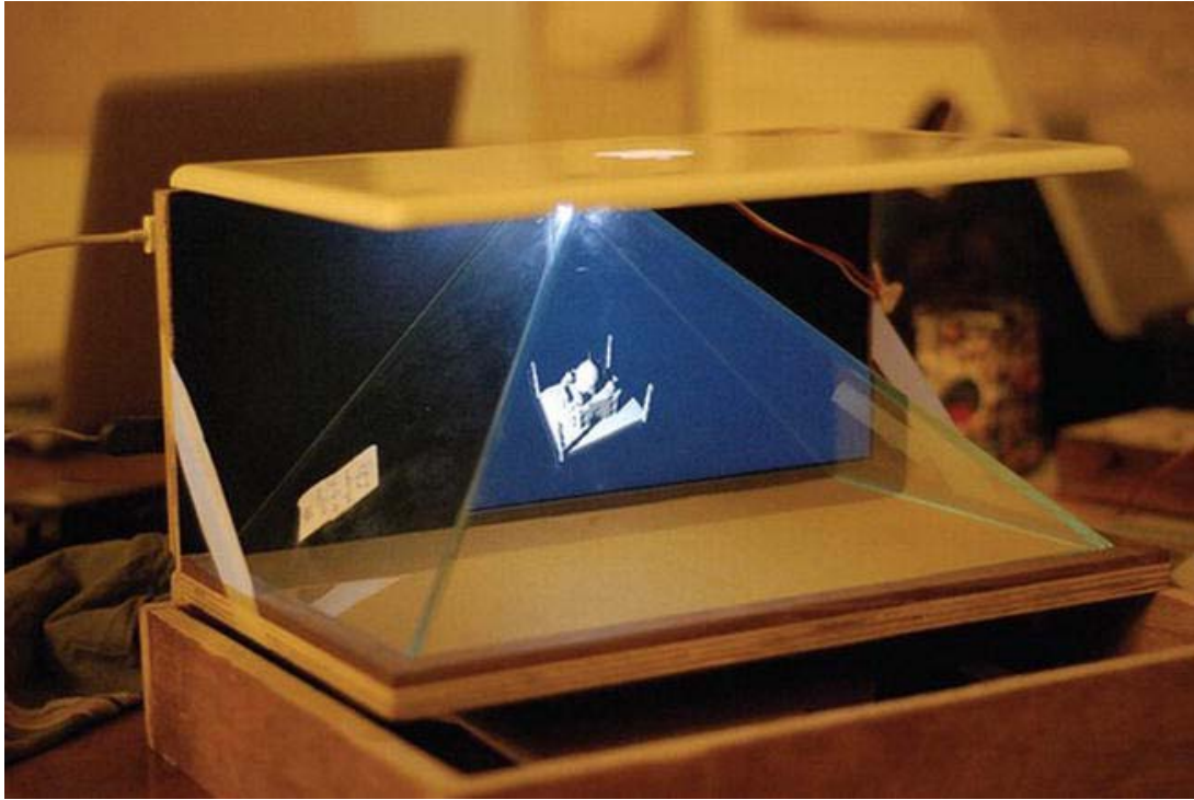
Figure 9-6. Three-pane Pepper's Ghost display with MacBook. Photo courtesy Ujjval Panchal
