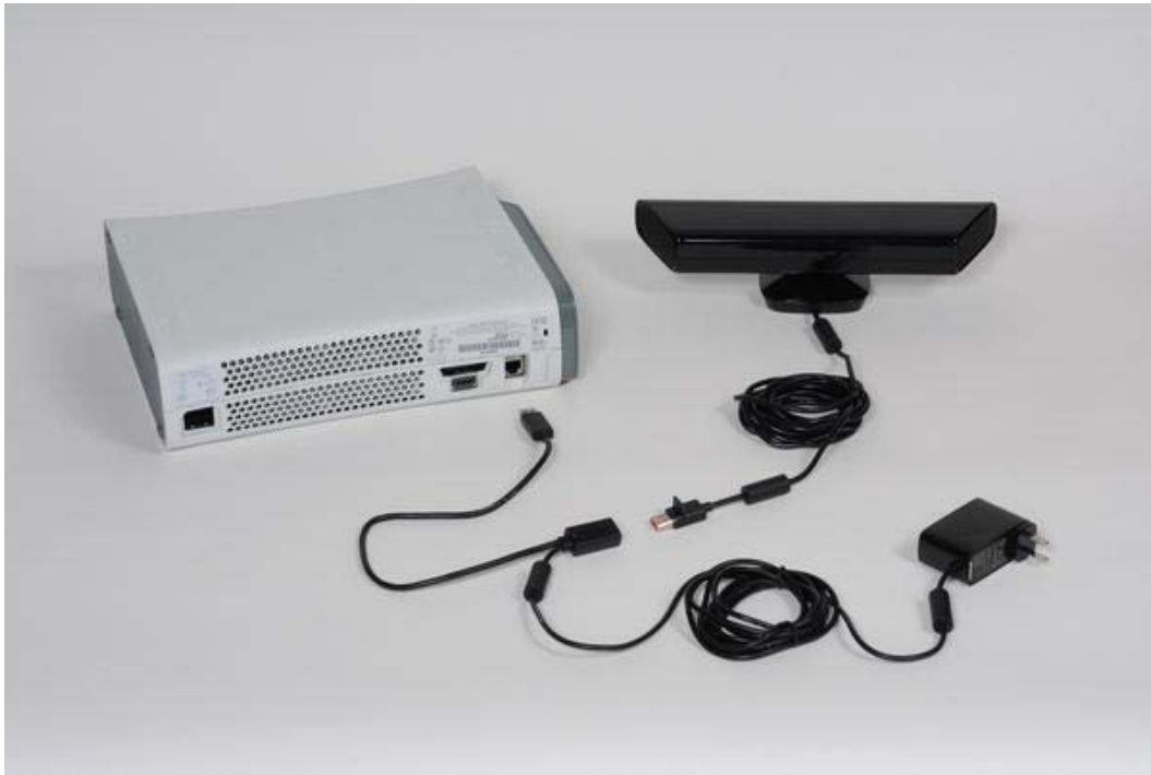
Figure 1-3. Unplugging the Kinect and AC adapter from an early model Xbox game console (Photo courtesy Microsoft)
