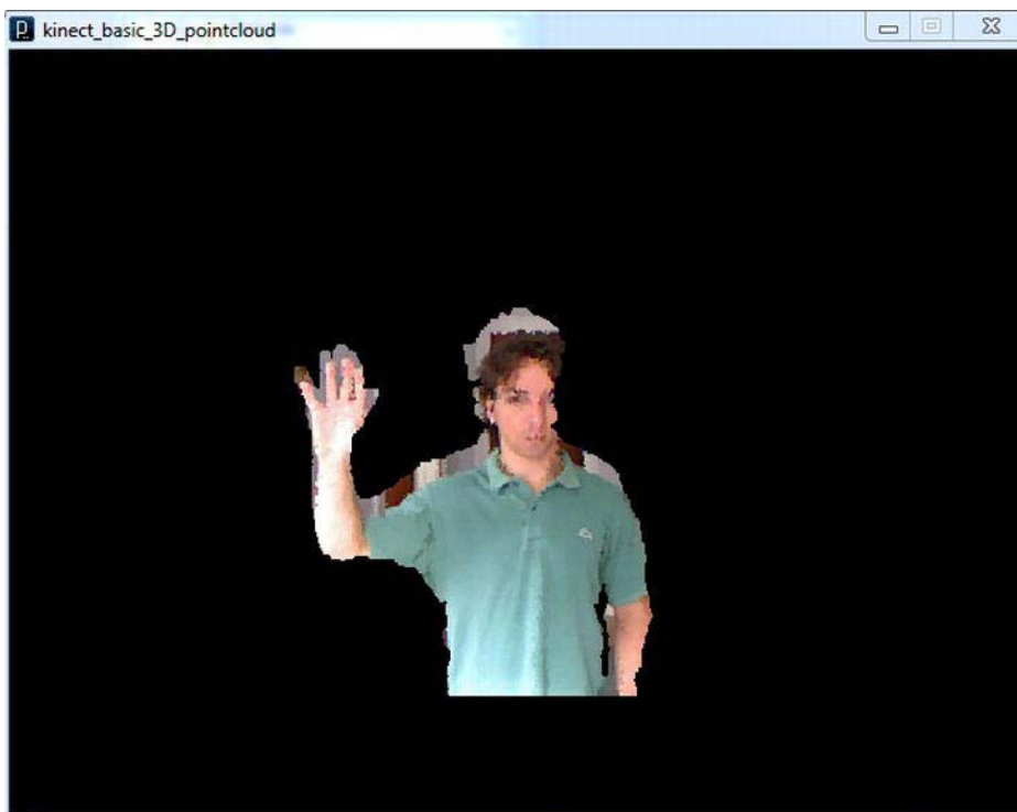
Figure 4-9. Thresholding example, with a poorly calibrated Kinect
