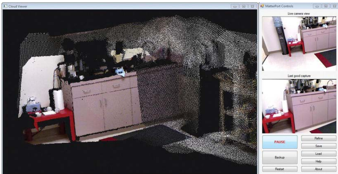
Figure 3-16. MatterPort capture in progress showing last good capture aligning with incoming capture information
