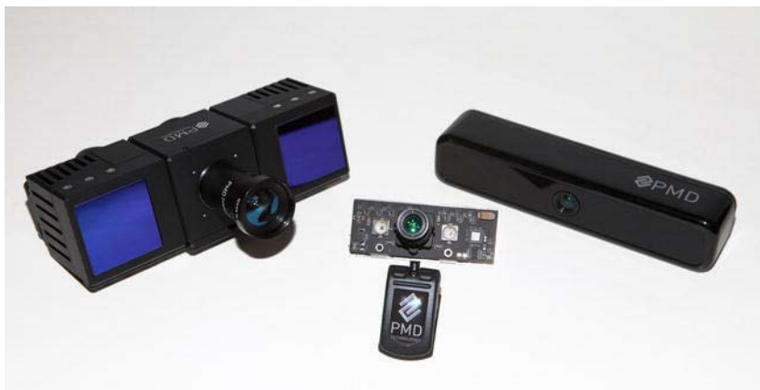
Figure 2-7. The PMD [vision] CamCube, PMD [vision] CamBoard reference design, and PMD [vision] ConceptCam. Photo by Kara Dahlberg.
