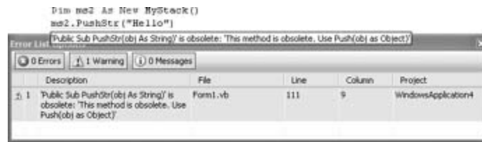
Figure 3-14. The Error List window displaying the warning on the obsolete method
