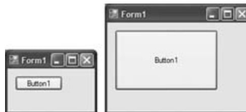
Figure 4-21. Setting the Anchor property of a control to "Top, Bottom, Left, Right"
