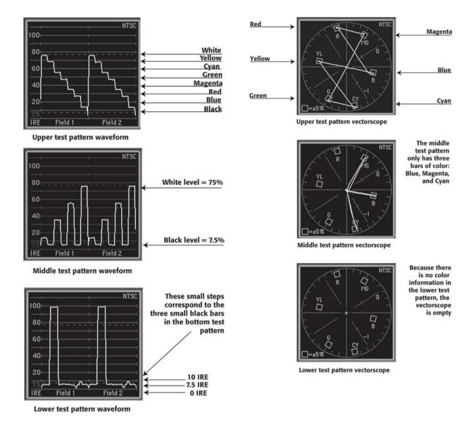
The waveforms (left) and vectorscopes (right) that correspond with the SMPTE color bars test patterns.
