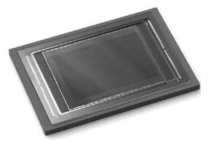
Single-chip cameras have red, green, and blue filters arranged over clusters of cells in the sensor. These filter the light coming through the lens and allow the camera to record color images. In a three-chip camera, a series of prisms split the incoming light into separate red, green, and blue components, and directs each of these components onto a separate sensor. Because the camera dedicates an entire sensor to each
