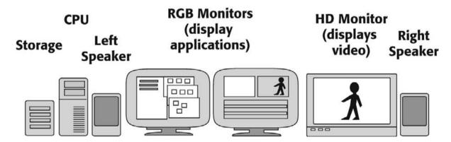
**Figure 11.1**Components of a typical tapeless HD editing workstation.
