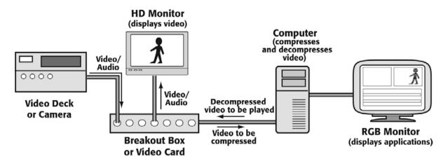
**Figure 11.4**Components of a typical SDI-based editing workstation.
