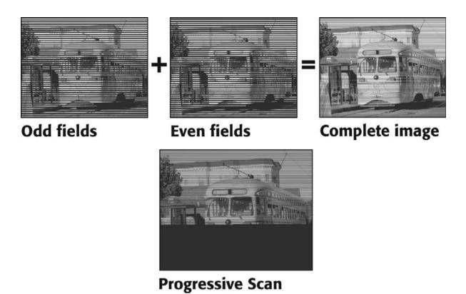
**Figure 3.2**Interlaced video uses two fields to make up a complete frame of video; progressive scan video does not have fields.
