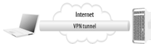
Figure 5-1. A tunnel established between two computers in a VPN
