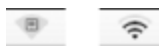
Figure 8-2. The icon of the AirPort in peer-to-peer (left) and infrastructure mode (right)
