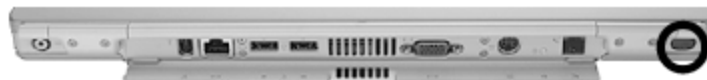
Figure A-3. The IR port (circled) on a PowerBook G4 (Gigabit Ethernet)
