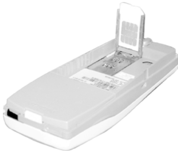
Figure 7-3. A SIM card inserted into a mobile phone
