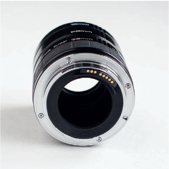
Three extension tubes attached together. These are 12 mm, 28 mm, and 36 mm extension tubes. An advantage to extension tubes over close-up filters is that they attach to any focal length lens and can be used separately or stacked together to make even closer micro views possible. They don't degrade image quality because they are hollow, and they connect to the camera's electronics so your meter still operates. When using extension tubes, you'll want to use a sturdy tripod and you might want to use your camera's mirror lockup, if the option is available, to prevent camera shake (covered in Chapter 5). If mirror lockup isn't an option, a self-timer or cable release is helpful. Fine focusing is a must, because depth of field is very shallow (covered in Chapter 4), so take your time and focus carefully.
