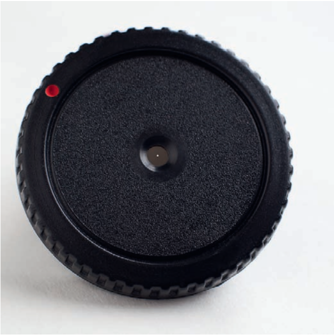
Pinhole body cap. Prefabricated pinholes (like this one) use a laser to drill a perfectly round aperture with sharp edges at a precise diameter optimized for the local length. This renders a sharper image while still having the other attributes of a pinhole camera. However, many photographers prefer to make their own pinholes, because the lack of precision adds welcome softness and unexpected attributes to its images.
