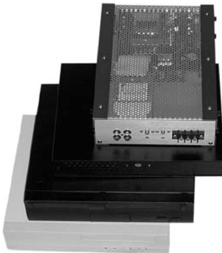
Morex (<http://www.morex.com.tw>) cases are some of the cheapest. They adapt easily to in-car use but don't have any car-specific power connectors, so power wires will have to pass through some hole into the case.
