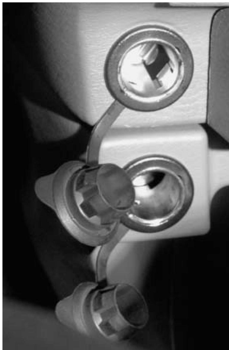
Unswitched outlets and hardwired accessories are always connected to the car's battery, whether the car is off or on. Car alarms are all wired this way, which is why they are designed to draw very little power. If you've ever left your lights on and come back to find that you can't start your car, you know why low power draw is important.
