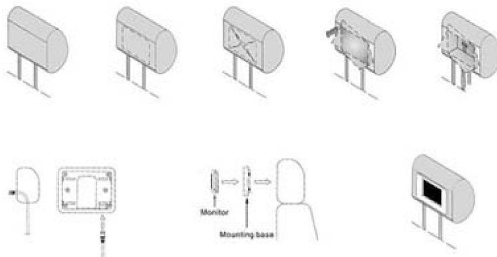
You won't be cutting a rectangle to install the frame. Instead, draw an X from corner to corner in the square you've drawn. Once you're sure the square is in the right place, take a razor blade or knife and cut along this X, so that you have four triangular flaps to fold out.
