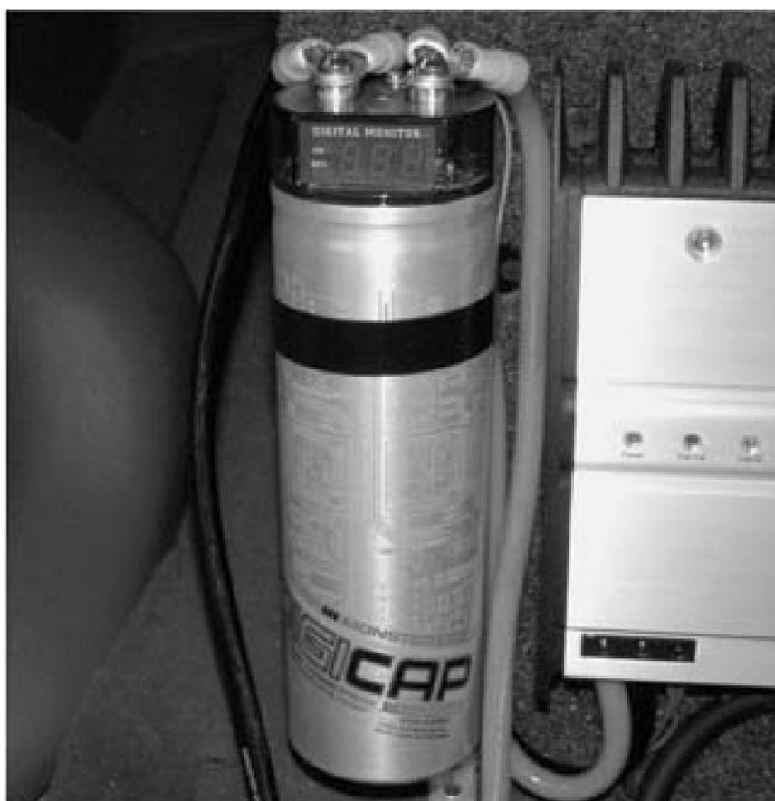
The 12V line from the battery (red/switched or yellow/unswitched) goes to the + side of the capacitor, and the ground (usually black) wire from the battery ground goes to the - side of the capacitor.
