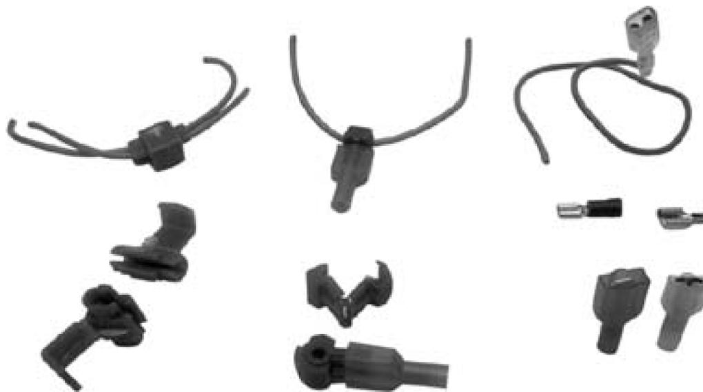
Another excellent crimp connector is a female blade plug tap ([Figure 1-13](#), middle). This connector crimps onto an existing continuous wire and forms a T outlet that a male blade connector can tap into. This is excellent, say, if you've found 12V and ground wires in the trunk of your Dad's Lexus that you want to use to plug in some device, but you want to be as inconspicuous as possible in case he decides to take the car back to the dealer after you've blown several fuses.
