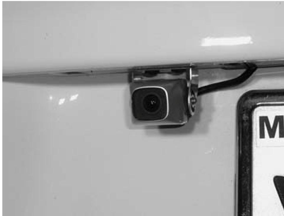
Figure 3-17. The watertight wire pipe, an important part of the wiring of your camera
