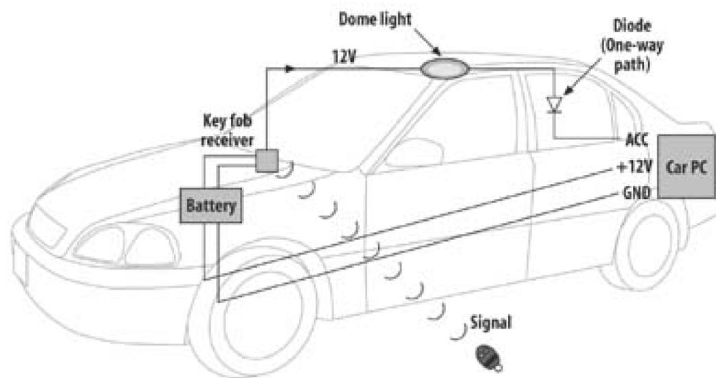
If you start blending different 12V trigger inputs to the car PC, such as dome light and ACC, *you must* use a diode between each input and the startup controller to ensure the voltages don't "backwash." Otherwise, the dome light may come on whenever the car is on, or the car radio may try to power up whenever the door opens. [Figure 4-15](#) shows how you can do this.
