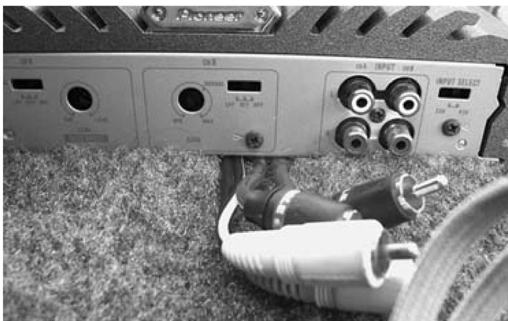
Figure 2-9. Adding an amp to the sound path
