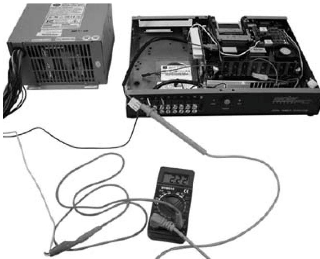
In our example, the computer is drawing around 2A. Our 50-Ah car battery could probably power this device for more than a day.
