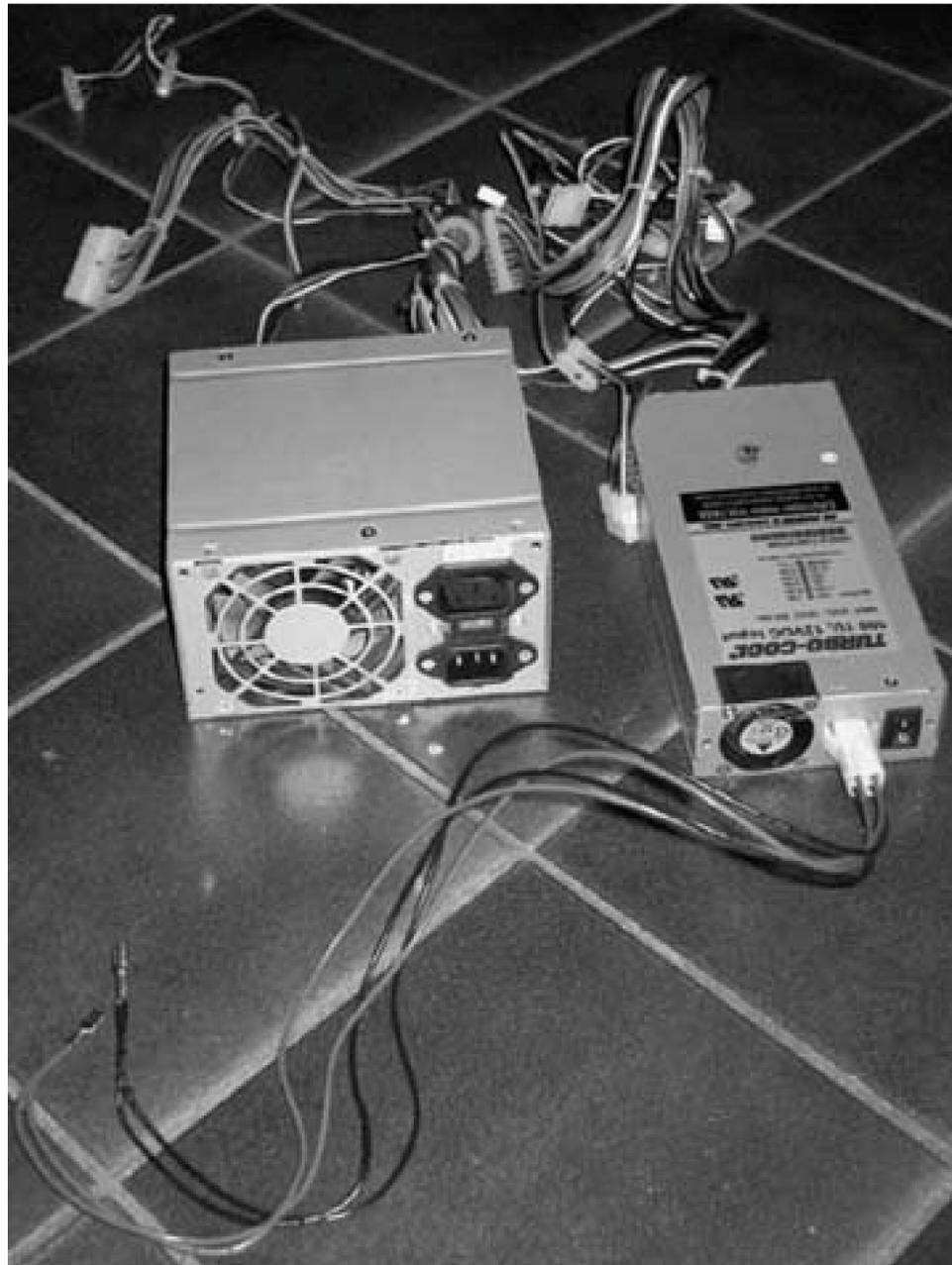
The power supply is controlled by the power-on signal from the motherboard, which has an idle current of about 100 mA. Accidental draining of the battery is not much of an issue, since this current is comparable to the idle current of other devices in the car (such as the alarm and the engine controller).
