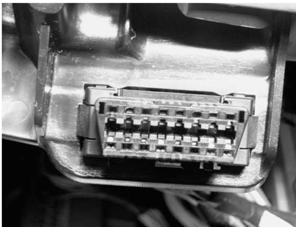
The functions of the different pins in the OBD-II connector are shown in [Table 7-1](#).
