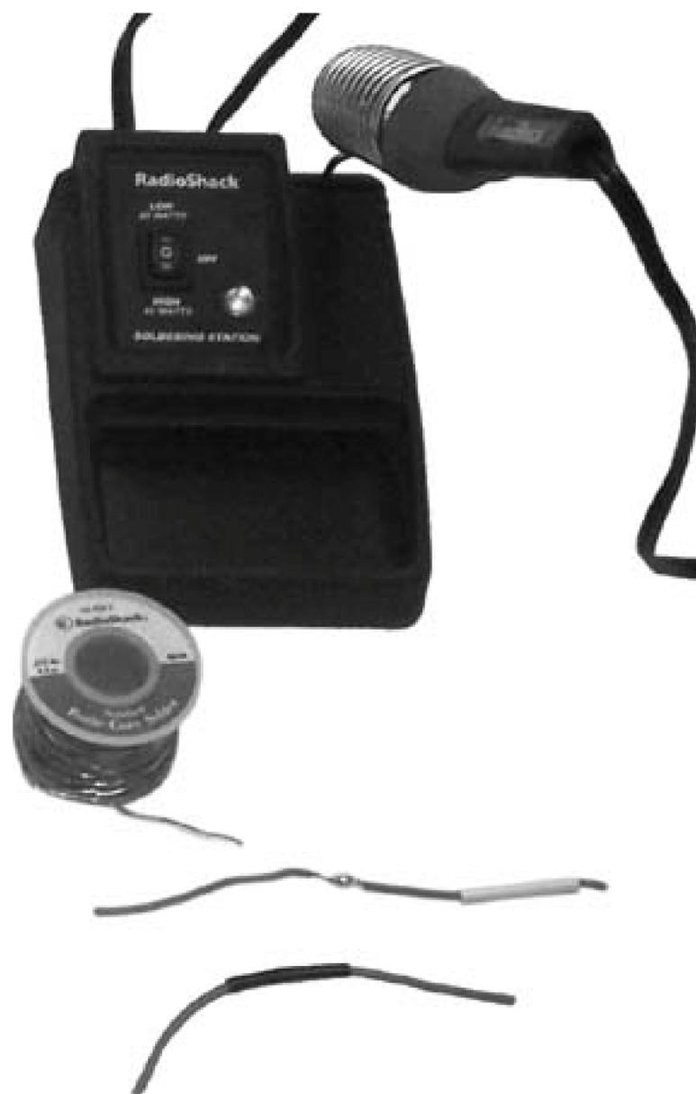
While this is no mini-course on soldering, the basic concepts here are that, being careful not to burn your hands, you place the two wires together, *heat them up*, and then put the solder on the wires. It will flow between all the wires (if they're braided) and make a nice solid bond.
