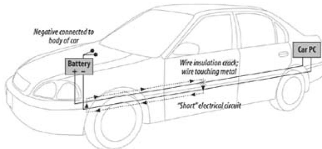
To protect against this situation, a fuse of a specific amp rating is put in the line between the battery and the device it powers, close to the battery itself. If a short circuit develops in the wiring or if the device malfunctions, the fuse simply melts once the amps get too high.
