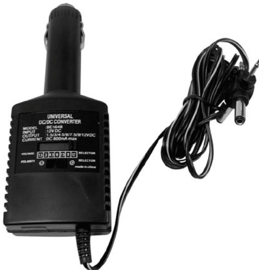
The second thing to determine is whether your device wants too much current. Any power adapter you purchase should specify a maximum amperage at which it will run, such as 1000 mA (1A). Any device you wish to power should have a corresponding amperage on its label, such as 800 mA. As long as the device's amperage is less than the maximum for the adapter, you can safely power the device.
