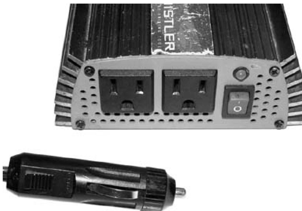
If you are using a smaller inverter, you are likely to quickly exceed its power, so you have to make sure you overcompensate. Also bear in mind that almost all devices have a current spike when they are first turned on or plugged in, so if you are using a small inverter at its wattage limit, you may need to power on your devices one at a time so as not to trip the circuit breaker or fuse built into the inverter.
