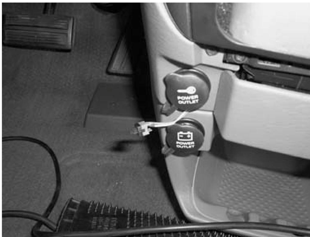
For my hack, I used two relays. One relay was connected to the accessory 12V of the vehicle; it closed one switch and opened another whenever the *car* was on. The other relay was connected to the 12V of the computer power supply; it closed one switch and opened another whenever the *computer* was on.
