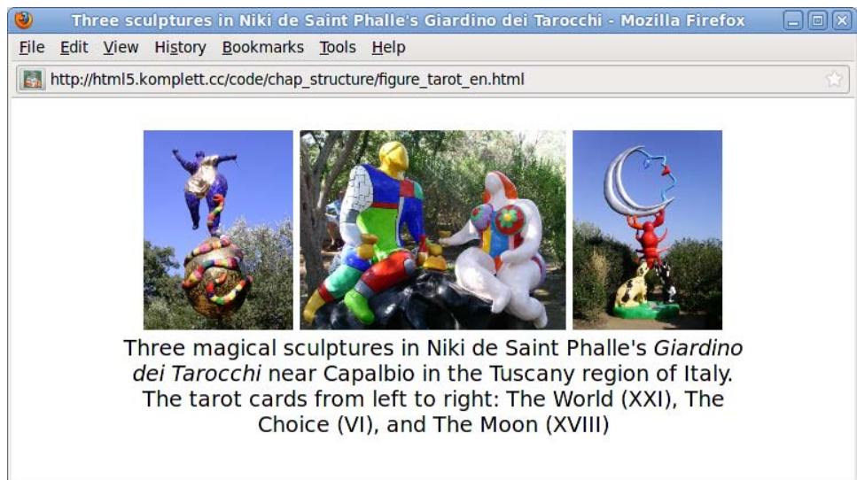
Figure 2.6 Example of “figure” with “figcaption”
