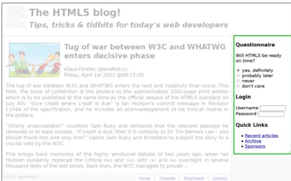
Figure 2.5 The basic structure of the HTML5 blog sidebar
