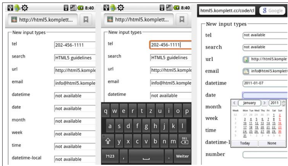
Figure 3.3 Support of new form input types on an Android 2.1 phone with browsers WebKit (left, center) and Opera (right)
