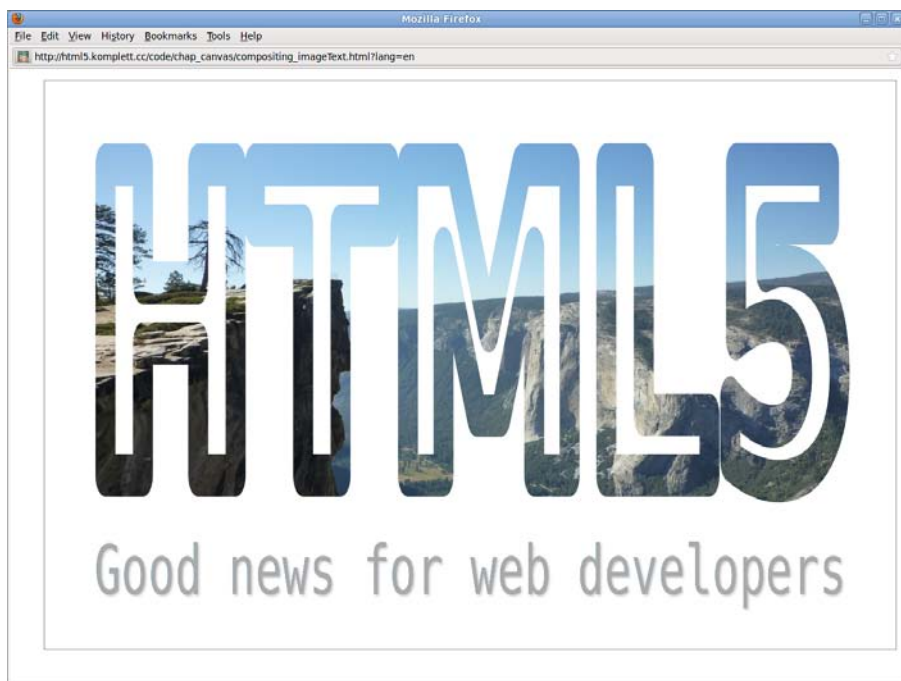
Figure 5.31 Compositing operation “destination-in” with image and text
