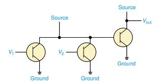
The NOR gate is the inverse of the OR gate, and the inverse of the inverse is the original. Thus, the output from the NOR gate is input to a NOT gate, giving us the NOR.
