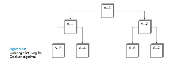
Eventually all the small sorted piles can be stacked one on top of the other to produce a sorted set of tests. See Figure 9.12.
