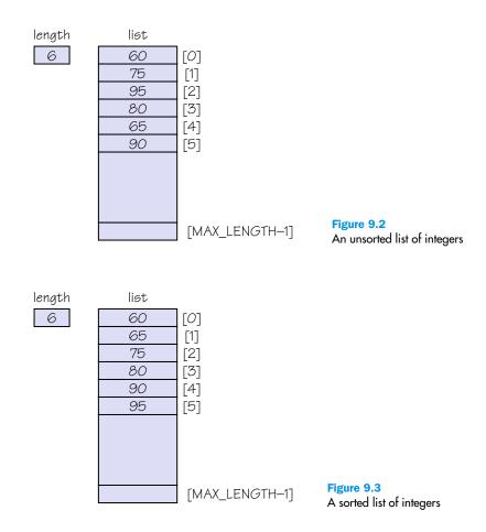
Get next item means to increment the value used as an index and access that indexed position.
