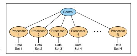
Figure 5.6 Processors in a synchronous computing environment
