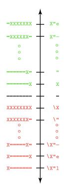
Addition and subtraction are accomplished the same way as in 10's complement arithmetic:
