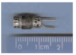
Figure 1.6 A transistor, replacing the vacuum tube Courtesy of Dr. Andrew Wylie
