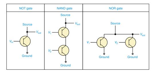
Figure 4.9 Constructing gates using transistors
