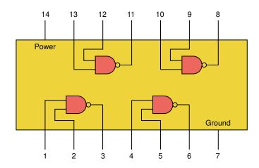
Integrated circuit (also chip) A piece of silicon on which multiple gates have been embedded
