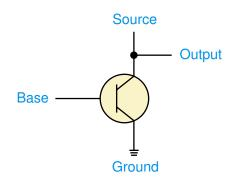
Figure 4.8 The connections of a transistor
