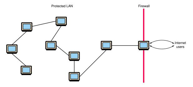
Figure 15.8 A firewall protecting a LAN
