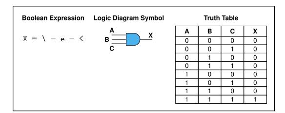
Figure 4.7 Various representations of a three-input AND gate
