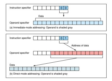
Figure 7.3 Difference between immediate-mode and direct-mode addressing
