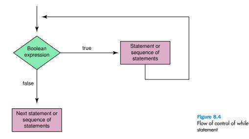
use of a special variable called a *loop control variable*. The first part is initialization: The loop control variable is initialized to some starting value. The second part is testing: Has the loop control variable reached a predetermined value? The third part is incrementation: The loop control variable is incremented by one. The following algorithm repeats a process limit times.
