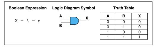
Figure 4.2 Various representations of an AND gate
