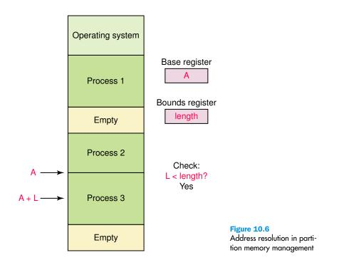
Base register A register that holds the beginning address of the current partition
