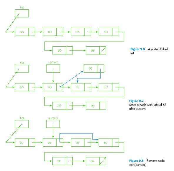
Put item means given current, insert a new node with item in the *info* part of the node between current and next(current). See Figure 9.7.
