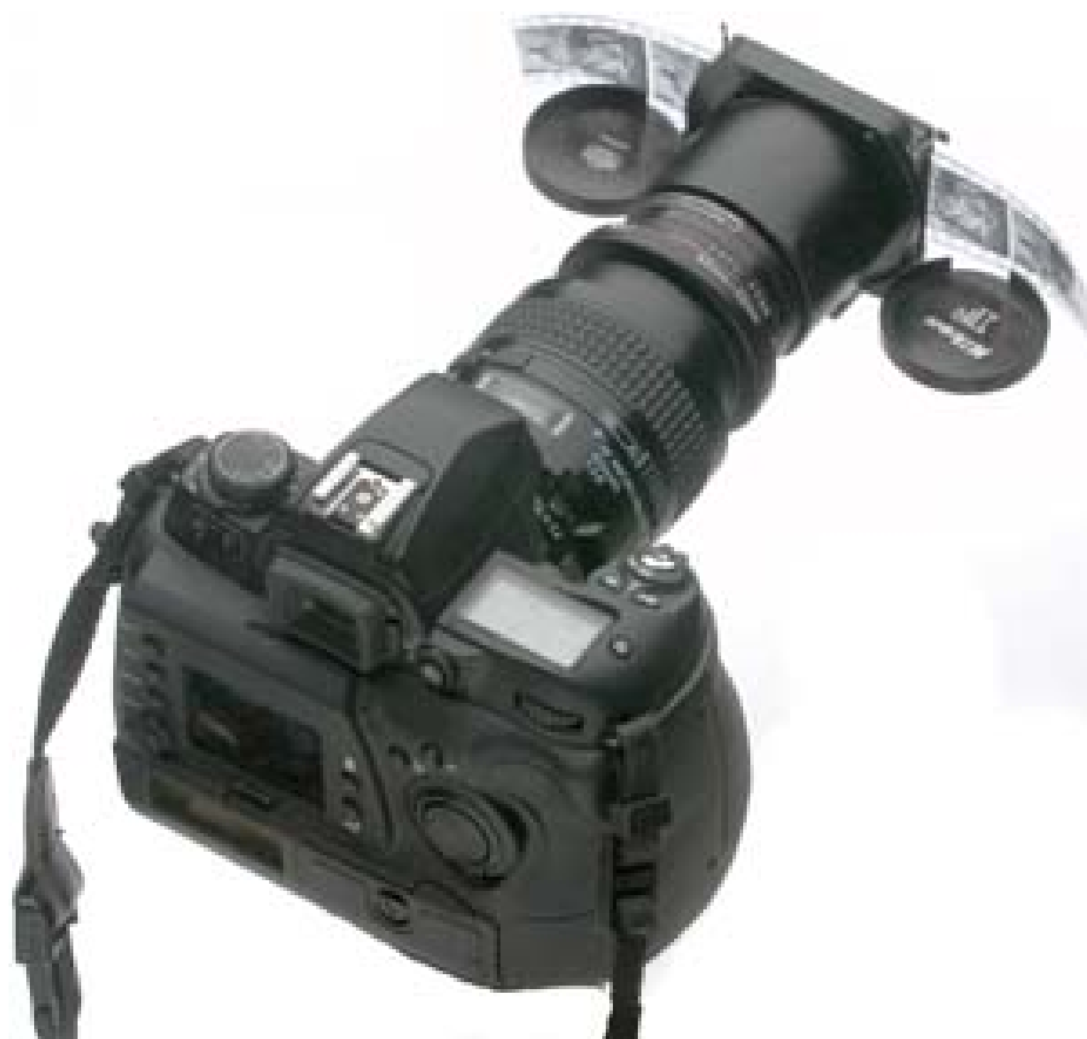
Figure 9-7. A digital camera with a copy attachment screwed onto a 60-mm macro lens.
