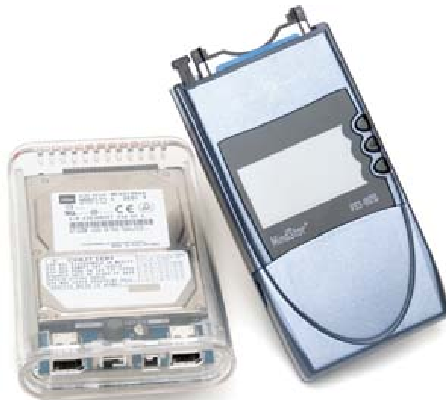
Figure 6-7. A "bus-powered" FireWire drive (it gets its power from the FireWire port, rather than from an external power supply) and a digital wallet.
