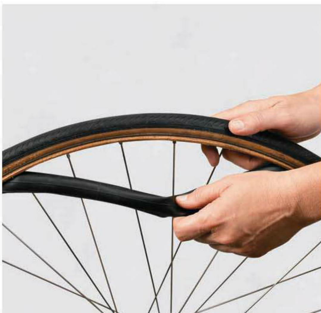
8 Remove the inner tube. It is not necessary to remove the tire except to fully inspect the inner lining of the tire and to inspect the rim tape.
