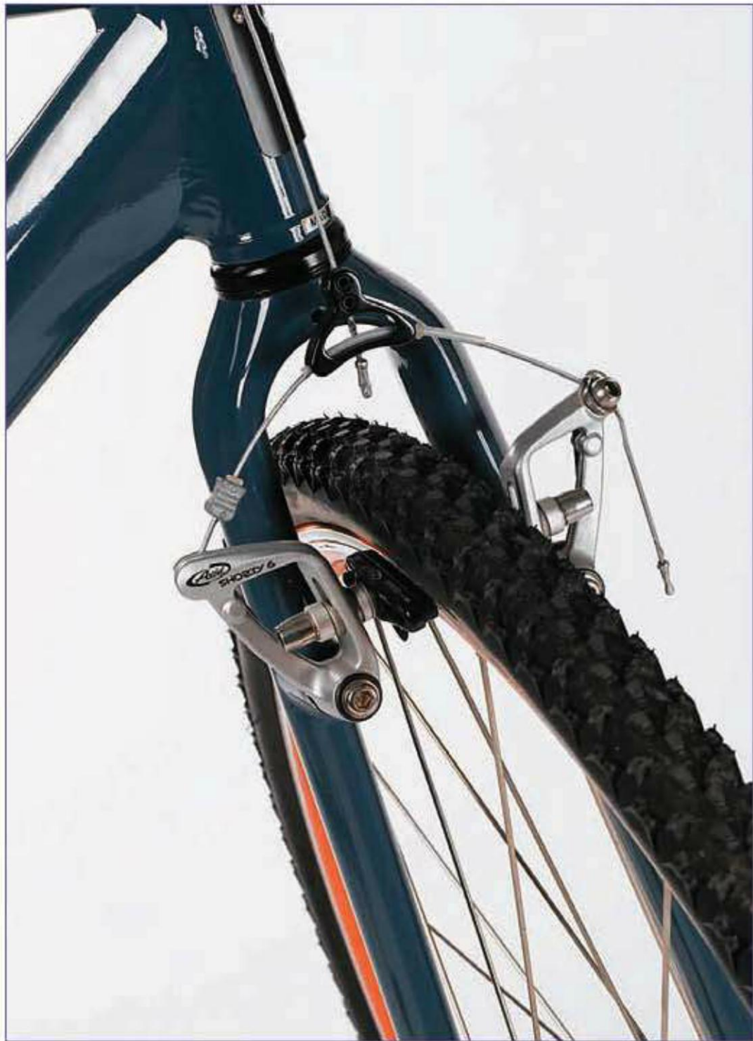
The cantilever brake has clearance for large tires and mud.
