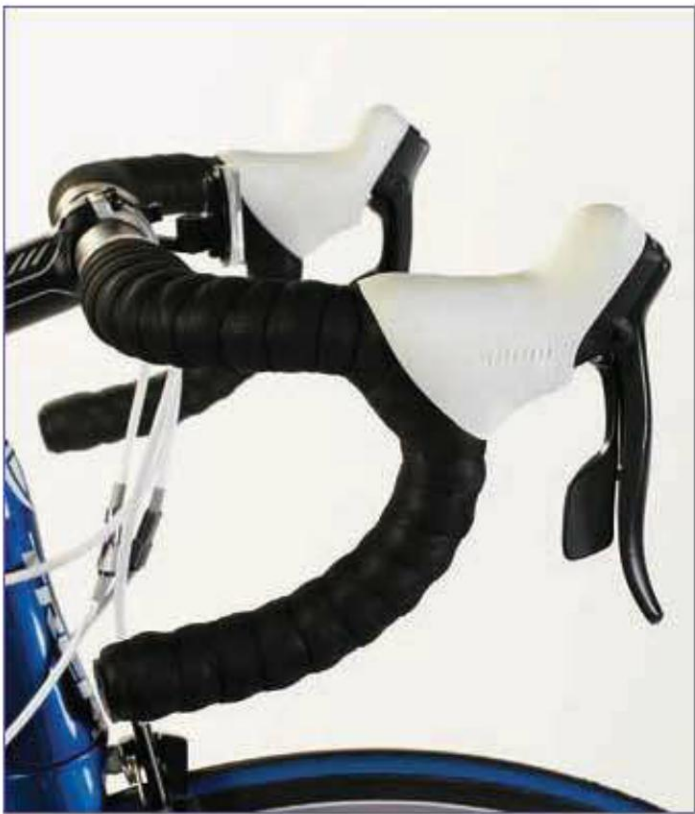
Most road bikes now have shift levers integrated with brake levers.
