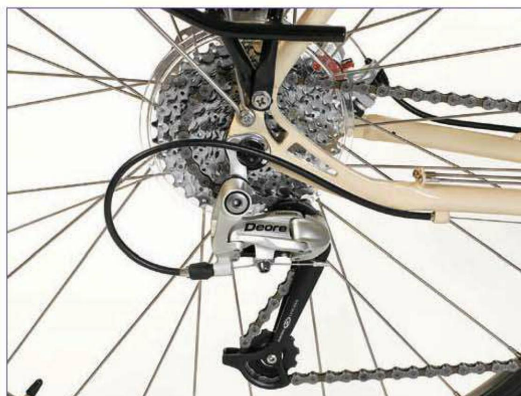
Mountain bikes and many hybrid and comfort bikes have a very wide range of gears. The cage on the deraillieur is longer to take up the extra chain length.
