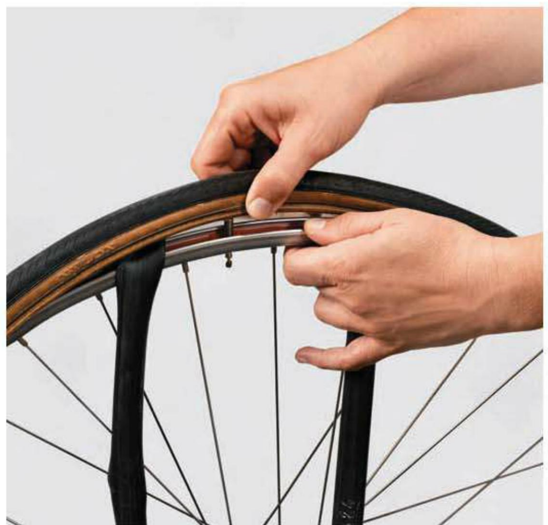
9 To remove the valve, push the tire back over the rim so you can pull the valve straight out to remove it.
