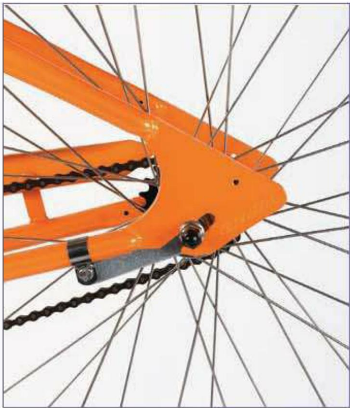
Coaster brakes are not affected by weather because they operate internally.
