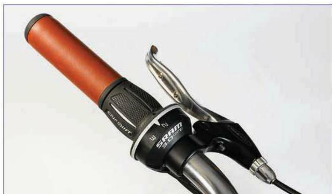
Twist shifters are easy to use and are always in hand, which is very safe.
