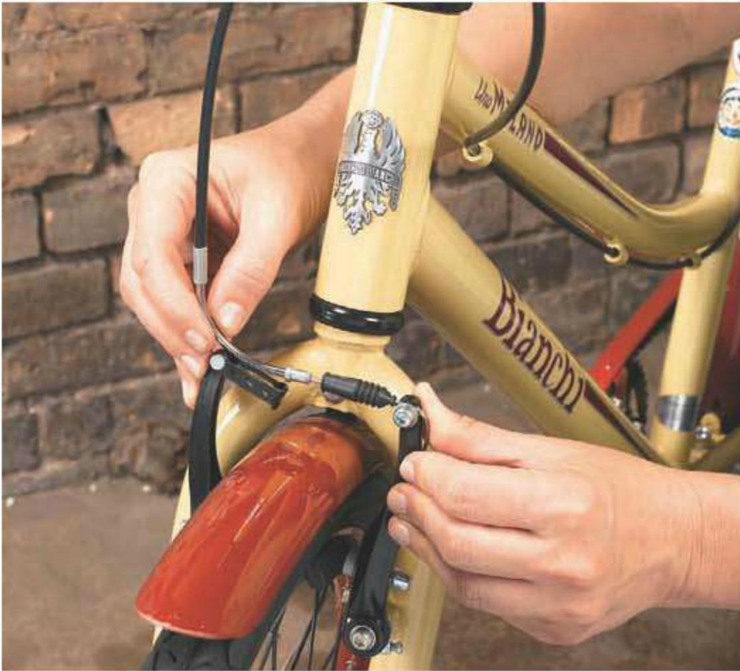
Linear pull brakes. Pinch the lever arms together at the top and lift the metal tube (noodle) out of the linkage bracket.
