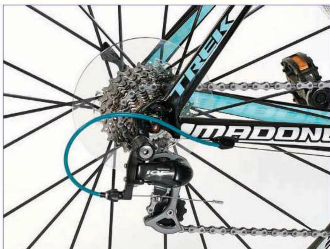
Most road bikes have a short cage deraillieur because the difference between the highest and lowest gears is small so there is not as much chain slack.
