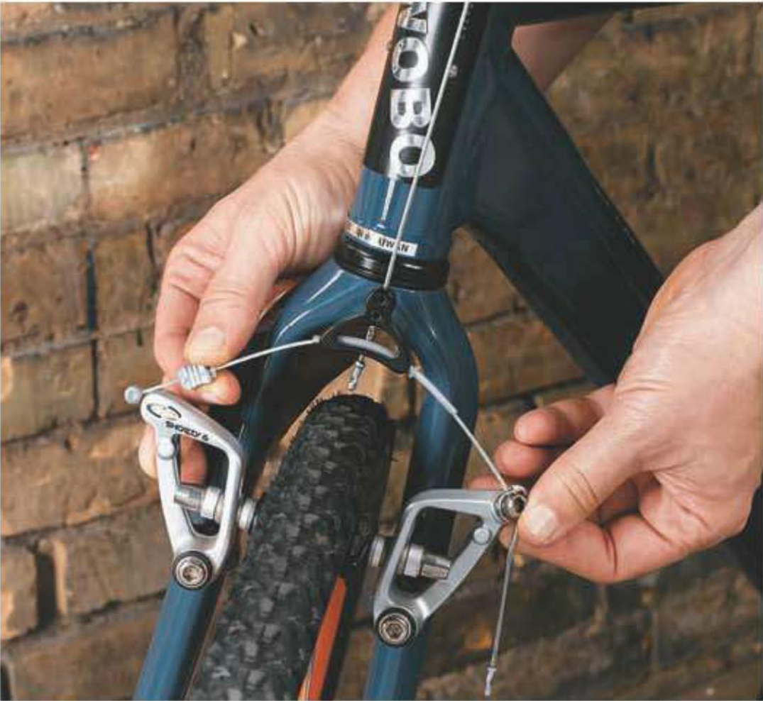
Cantilever brakes. Pinch the lever arms together at the top and remove the straddle wire cable.
