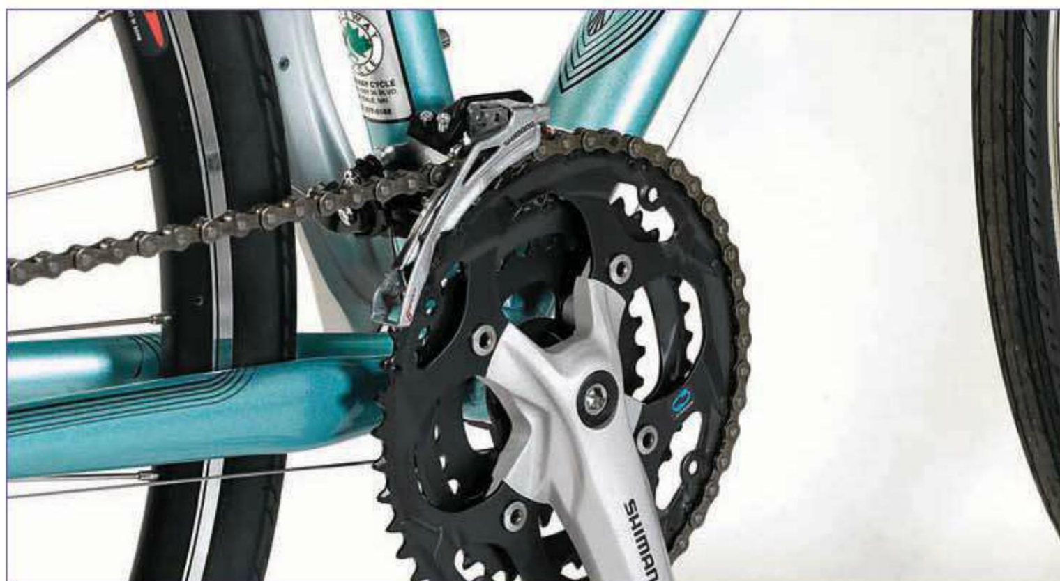
The front deraillieur pushes and lifts or drops the chain between chainrings.
