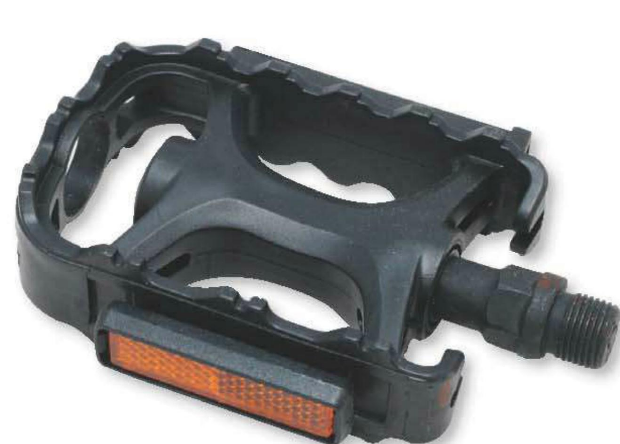
The classic bicycle pedal has grippy edges and rotates on its own axle after it is screwed to the crank arm.
