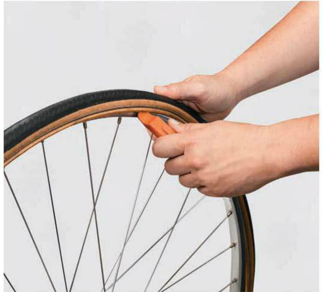
7 The tire should now be loose enough that you can run the tire lever around the entire tire and lift it over the rim.
