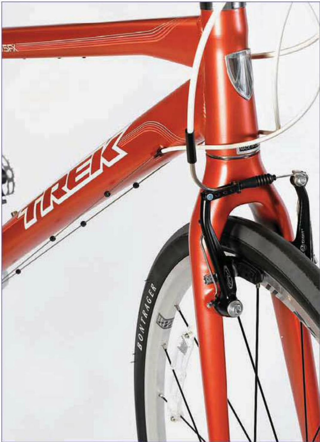
Linear pull brakes have good clearance and excellent stopping power.
