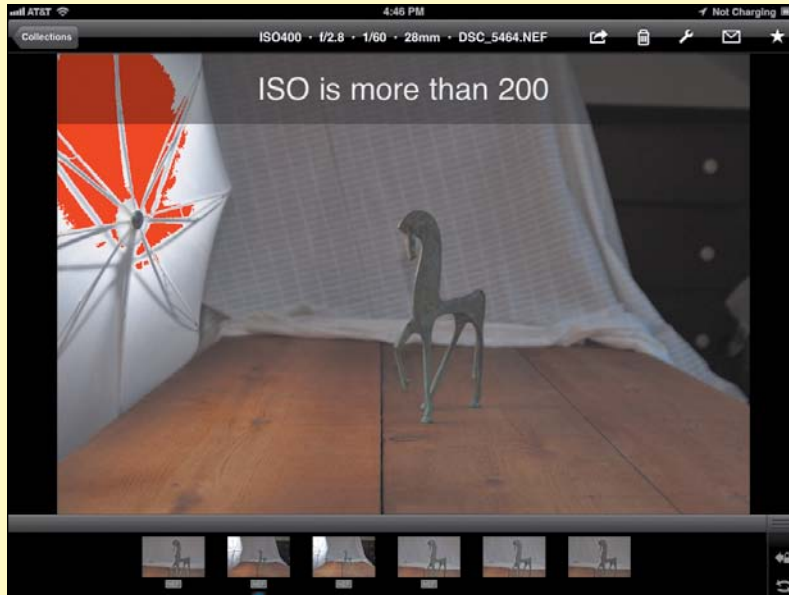
1.14 ShutterSnitch warns that my ISO is high and highlights hot areas of the photo (in red).
