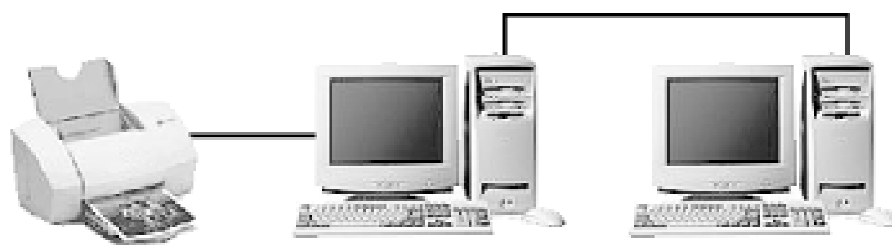
Figure 7-2. A quick-and-dirty hubless workgroup.
