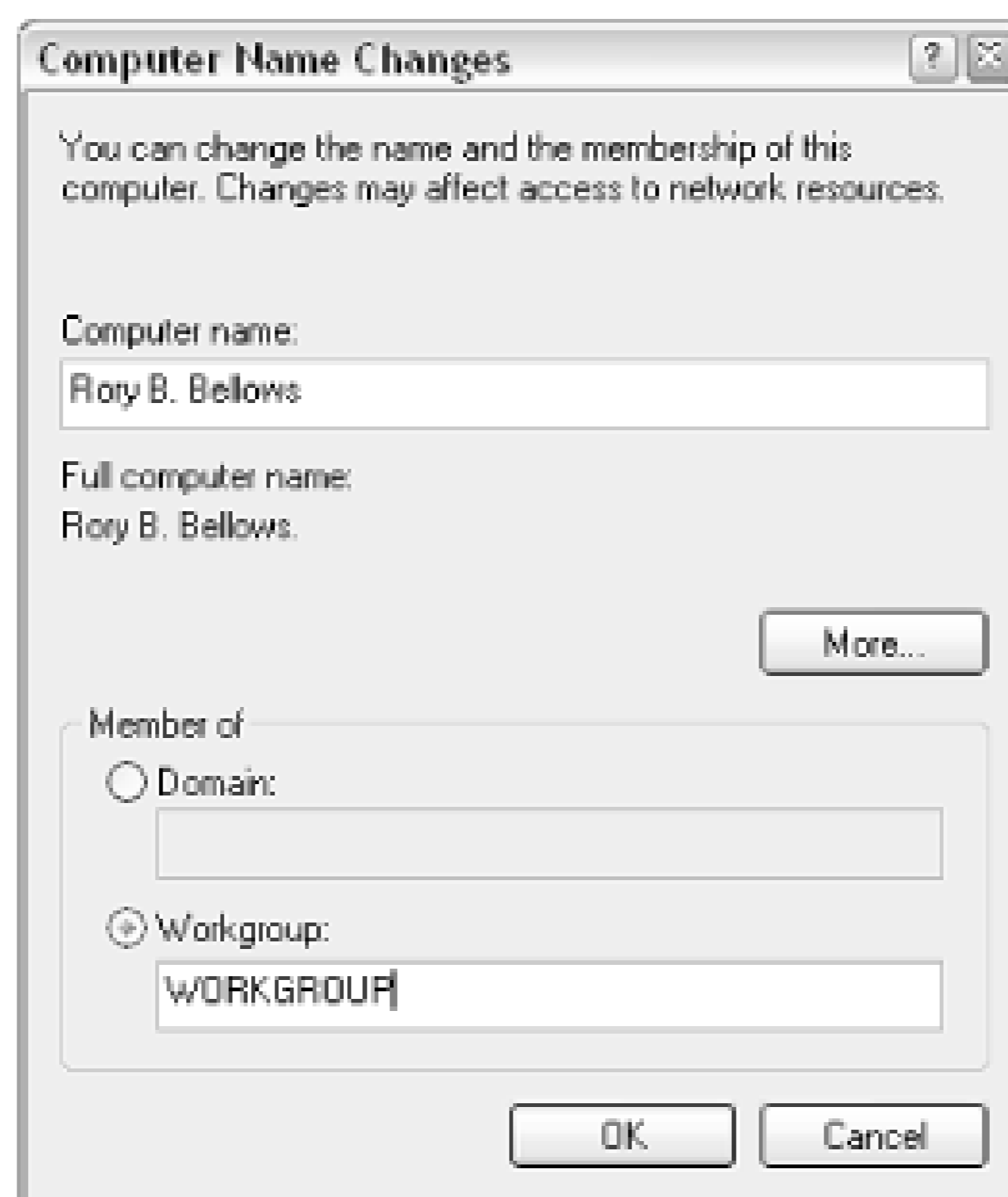
Figure 7-8. You'll need to open the Computer Name Changes dialog to identify your computer on your network.
