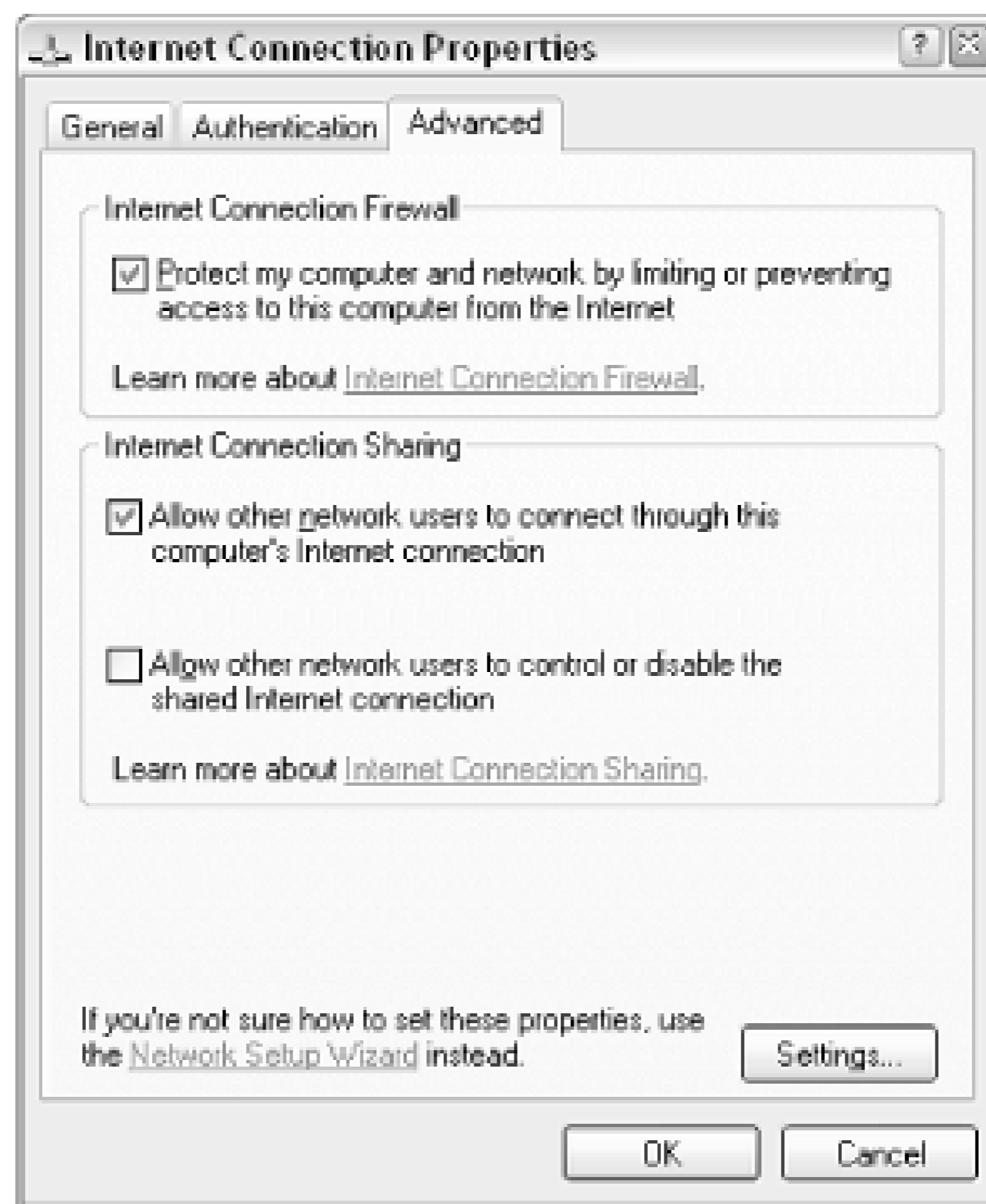
Figure 7-9. Any Internet connection can be shared with other computers in your workgroup.
