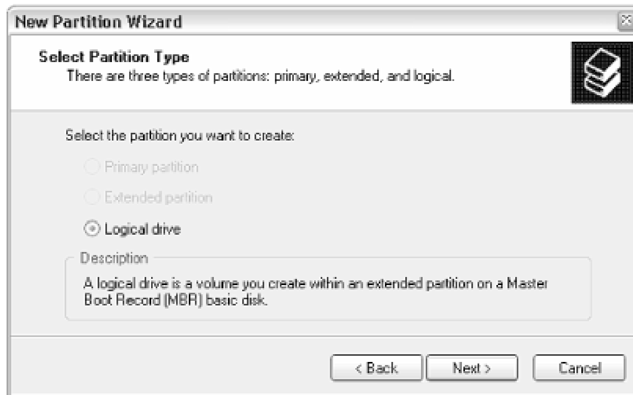
Figure 10-4. There are three basic types of partitions, each used under a specific circumstance.
