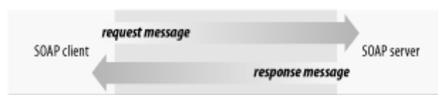
Figure 2-3. Basic RPC messaging architecture
