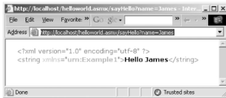
Figure 3-8. A typical HTTP-GET web service response
