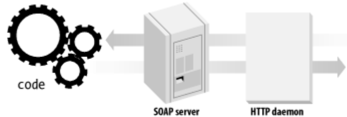
Figure 3-1. The HTTP daemon passes the request to the SOAP proxy, which then invokes the code behind the web service
