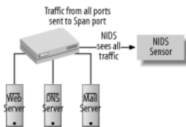
Figure 9-7. Span port on a switch
