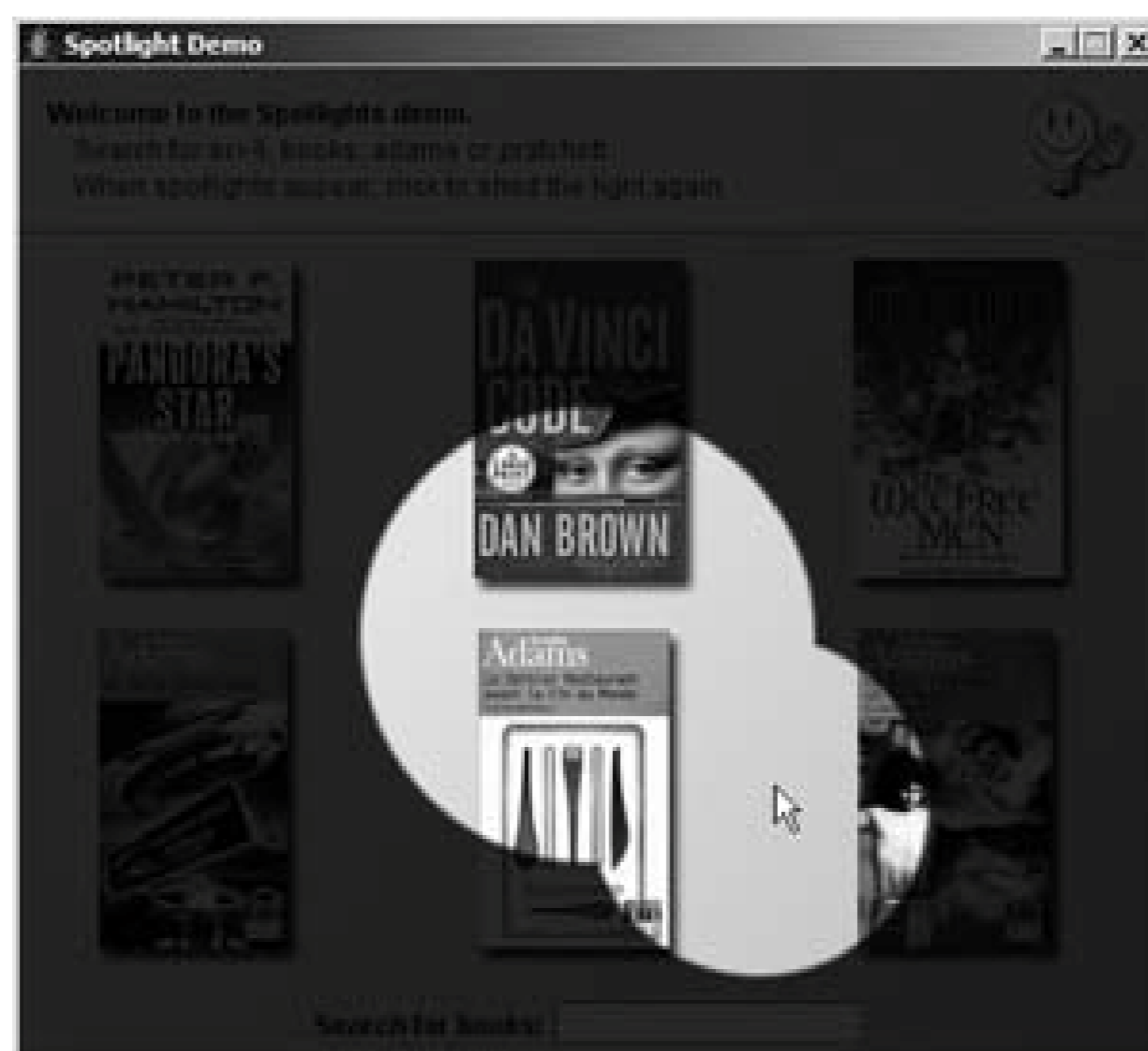
Figure 8-15. By subtracting ellipses to a rectangle, you can easily overlap the spotlights
