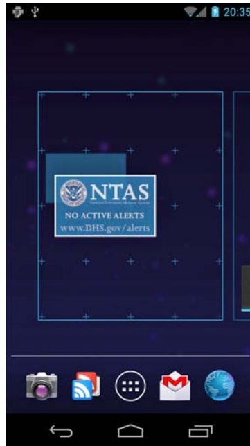
Figure 22.2 A simple App Widget being placed on the Home screen that displays NTAS alerts.
