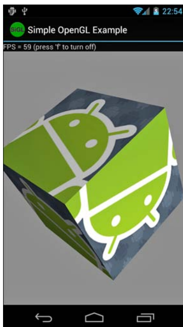
Figure 20.6 A textured, lit, shaded cube with the frame rate displayed.
