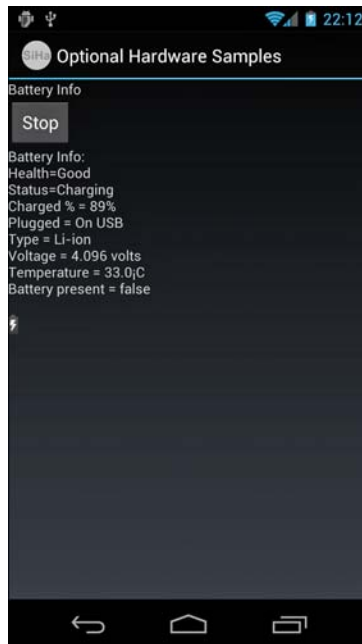
Figure 16.2 Screen capture showing values from the battery monitor from a physical device.
