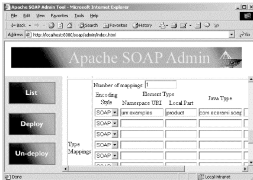
Figure 5-1. Deploying a SOAP service with a new type-mapping entry
