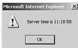
FIGURE 17.2 Returning the server time in XML via a POST request.
