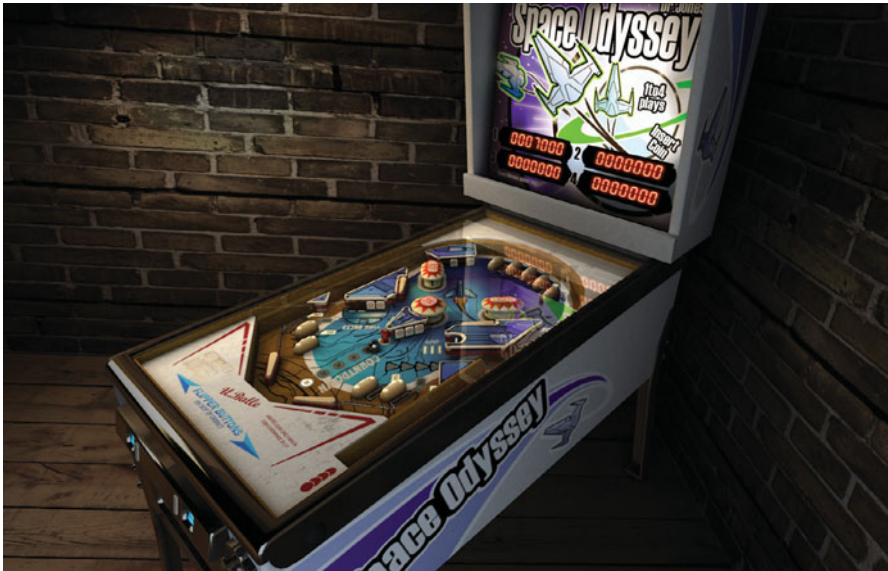
Color Plate 1 The OpenGL ES 2.0 Pinball Demo from AMD demonstrates the use of shaders for effects such as environment mapping and per-fragment lighting. (© 2008 Advanced Micro Devices, Inc. Reprinted with permission.)
