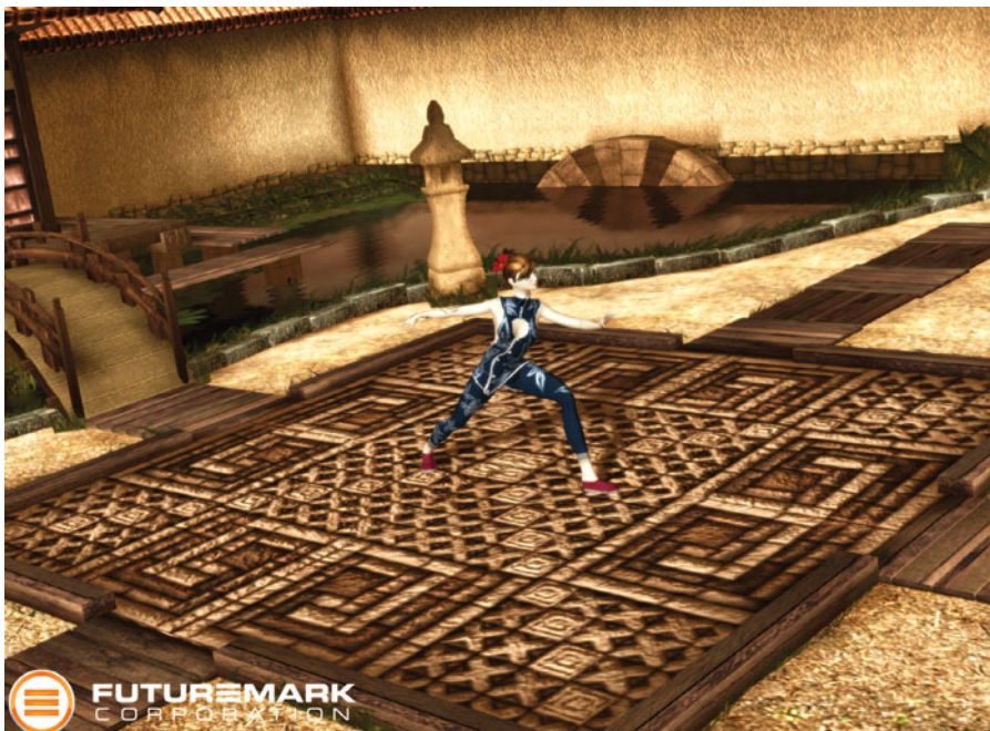
Color Plate 3 Screenshot from the Taiji scene in 3DMarkMobile ES 2.0 by Futuremark. The Taiji character is rendered using vertex skinning. Her shadow that is cast onto the ground by rendering to a depth texture bound to a framebuffer object and then using that depth texture as a shadow map.(Source: 3DMarkMobile ES 2.0 that is a trademark of Futuremark Corporation.)
